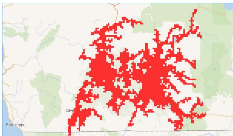
Medford (27 cust/line mile) PAC Trans Subs: 16 Cust Trans Subs: 1 PAC Distr Subs: 44 (22%) Cust Meters: 142,380 (23%) Svc Transformers: 49,365 (29%) Distr Line Miles: 5,315 (28%) 2 Distr Engineers 49% of circuits have SCADA
