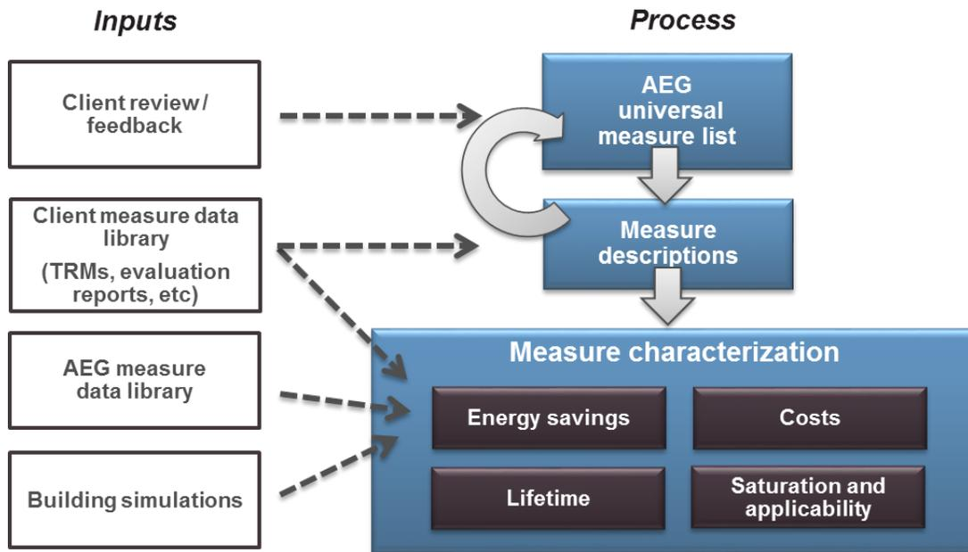
The framework for assessing savings, costs, and other attributes of energy efficiency measures involves identifying the list of energy efficiency measures to include in the analysis, determining their applicability to each market sector and segment, fully characterizing each measure, and preparing for integration with the greater potential modeling process.
