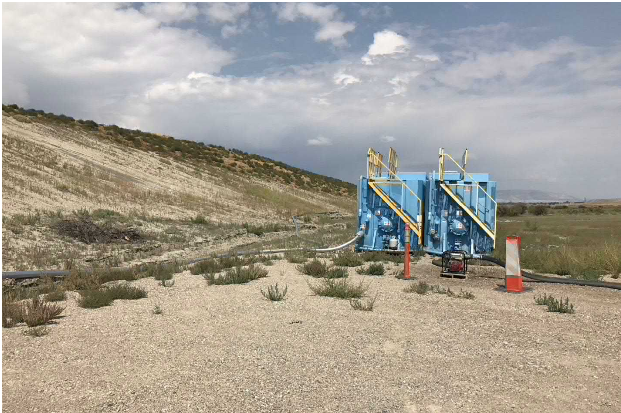
Photograph No. 27 View of Frac tank used for underdrain water storage, looking north-northwest.
