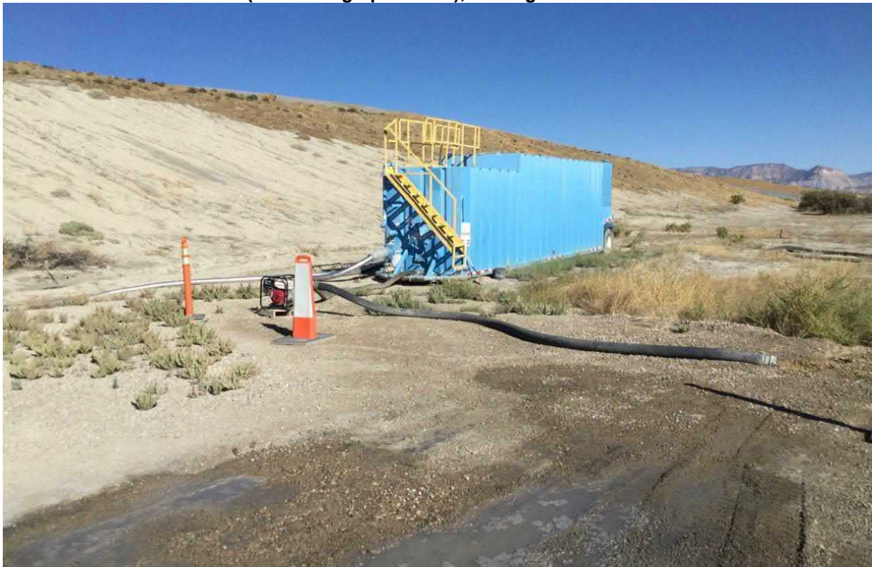
Photograph No. 20 View of Frac tank used for underdrain water storage, looking north-northwest.
