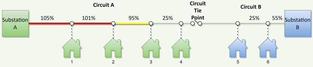
Solution: Upgrade wire to larger size to increase capacity rating
