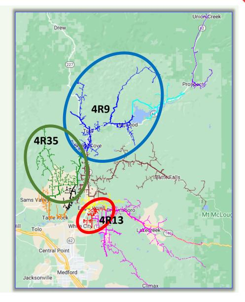
Planned load transfer of over 500 customer to 4R41 for sectionalizing purposes
