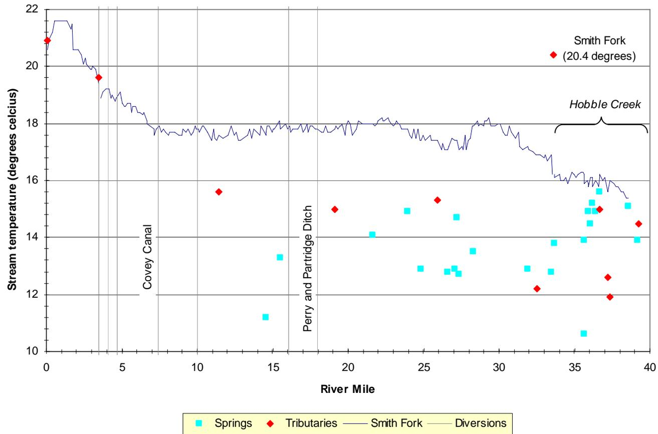
Figure 8 - Median channel temperatures plotted versus river mile for the Smiths Fork. The locations of detected surface inflows are illustrated on the profile and listed in Table 12.
