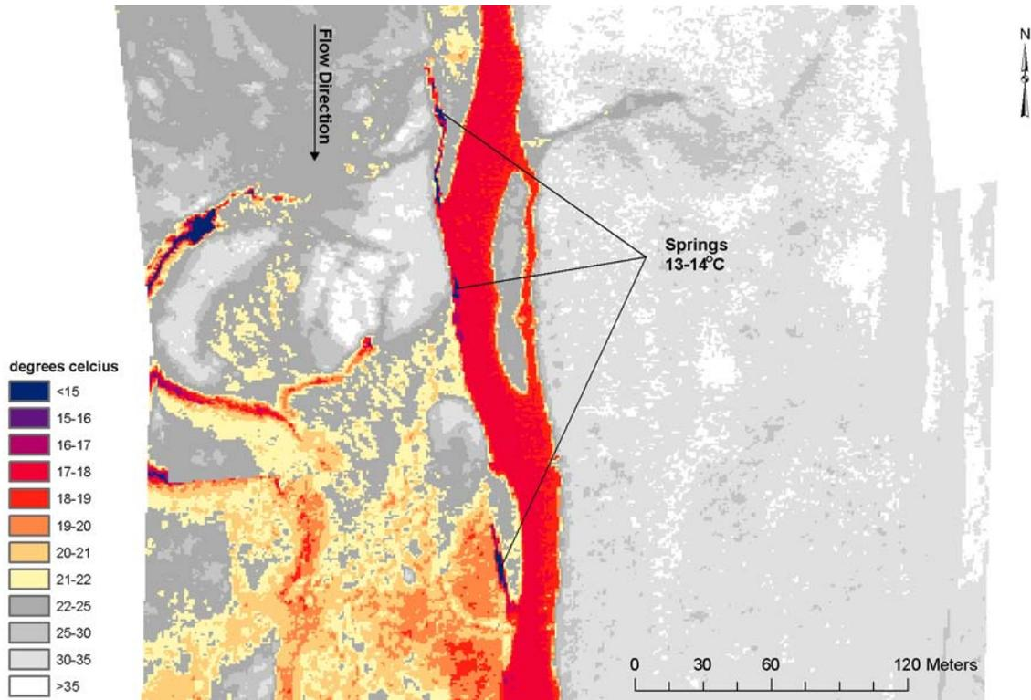
Smiths Fork Image 4. TIR image at river mile 28.3. A number of springs were detected between river mile 23.9 and 28.3, which appeared to contribute to lower main stem temperatures observed in this reach. This image shows three springs which drop the bulk temperature of the Smith's Fork from 18°C to 17°C.
