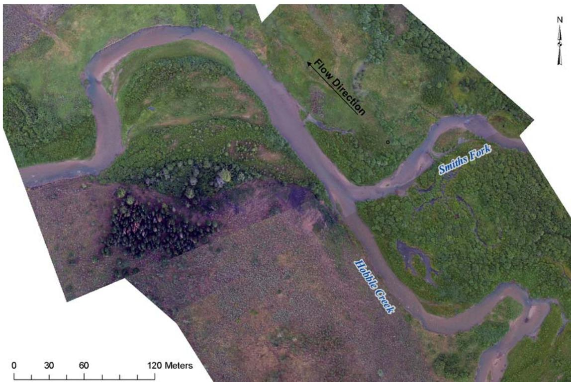
*Smiths Fork Image 3. TIR and true color image of river mile 33.55, Hubble Creek – Smiths Fork confluence. Radiant water temperatures at the mouth of Hubble Creek were  $\sim 16.4^{\circ}\text{C}$  compared to measured temperatures of  $20.4^{\circ}\text{C}$  in the Smiths Fork. The mixed water temperature was  $\sim 16.9^{\circ}\text{C}$  indicating that the flow from Hubble Creek sets the thermal regime of the Smiths Fork at this point.*
