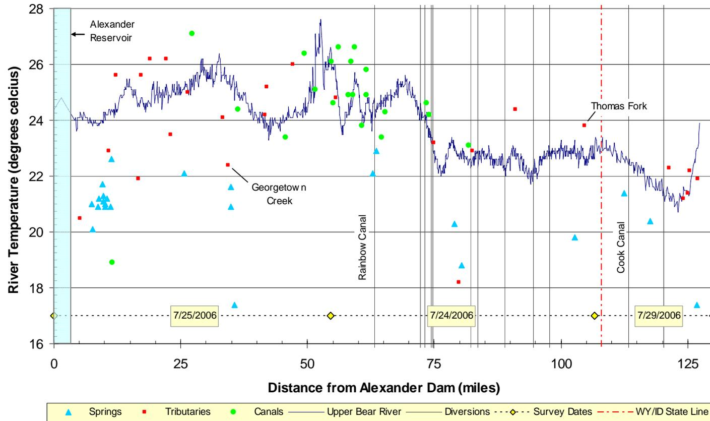
Figure 6 - Median channel temperatures plotted versus river mile for the Upper Bear River. The locations of detected surface inflows are illustrated on the profile and listed in Table 10.
