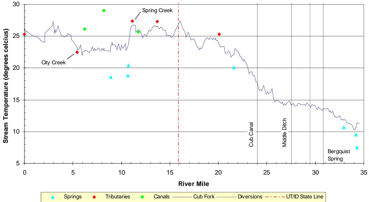
Figure 7 - Median channel temperatures plotted versus river mile for the Cub River. The locations of detected surface inflows are illustrated on the profile and are listed in Table 11.
