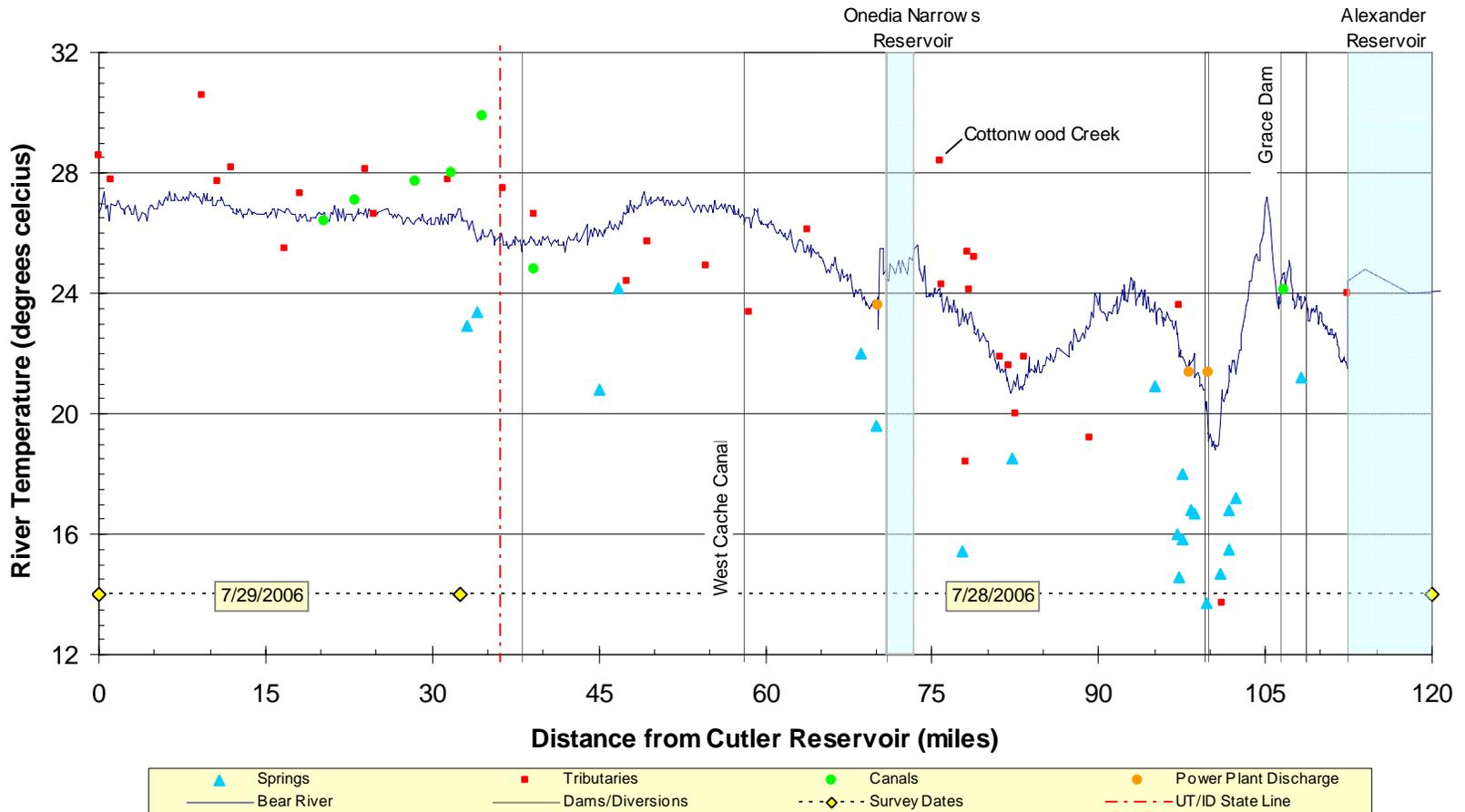
Figure 5 - Median channel temperatures plotted versus river mile for the Lower Bear River. The locations of detected surface inflows are illustrated on the profile and listed in Table 9..
