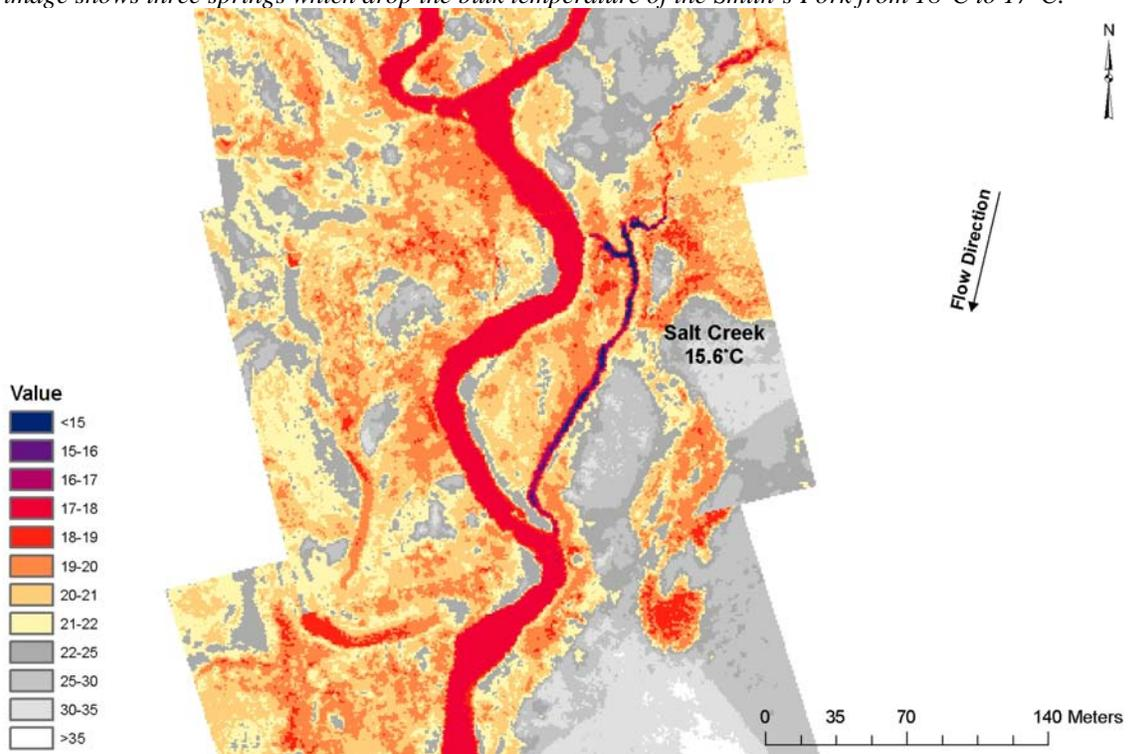
Smiths Fork Image 5. The TIR image shows the inflow of Salt Creek into the Smiths Fork at river mile 11.4. Even with two cold tributaries and three springs, radiant water temperatures in the Smiths Fork remained relatively constant (i.e. 17.4°C to 18.2°C) between river mile 23.4 and 6.9.
