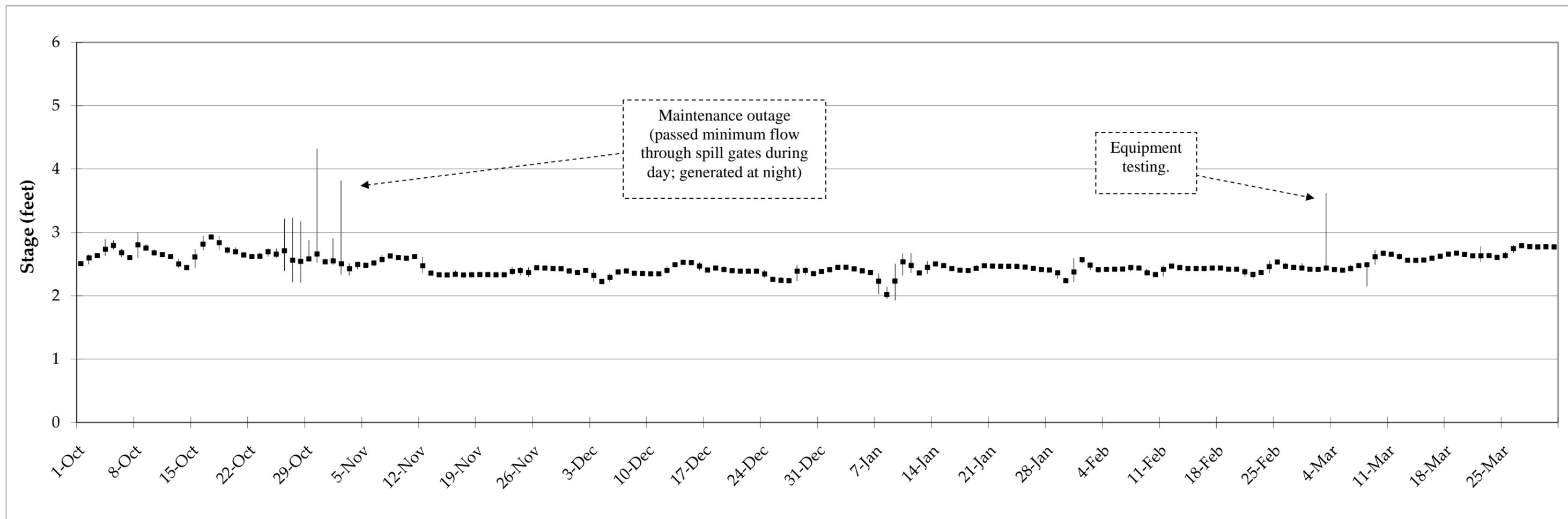
**Figure 3.** October 2009 through March 2010 daily average, maximum and minimum stage below Oneida. Precise values for each day and explanations are provided in Appendix A. Corresponding flows are shown in Figure 1.
