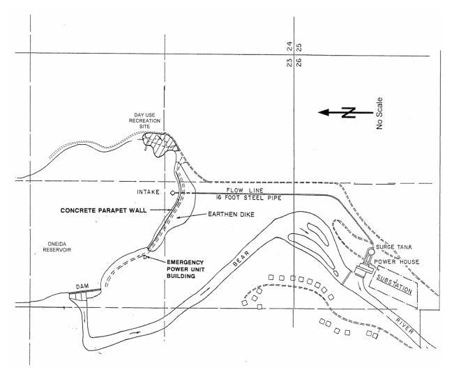
Figure 2-1. Oneida Project schematic showing main Project components (source: PacifiCorp Bear River FERC No. 20).
