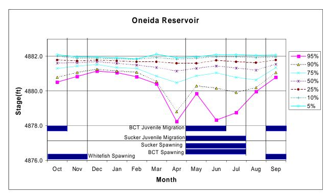
Figure 3-2. Percent exceedence curves for Oneida Reservoir stage readings with fish passage seasons shown (stage reading data source: Unpublished data PacifiCorp 2000-2009).
