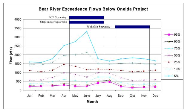
Figure 3-3. Percent exceedence curves for flows below the Oneida Hydroelectric Project with fish passage seasons shown (flow data source: Unpublished data PacifiCorp 1914-2009).
