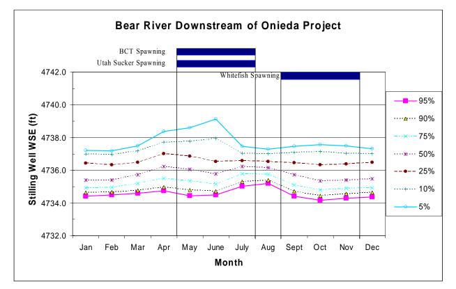
Figure 3-4. Stilling well water surface exceedence elevations below the Oneida Hydroelectric Project with fish passage seasons shown (flow and stilling well rating curve data source: Unpublished data PacifiCorp 1914-2009).
