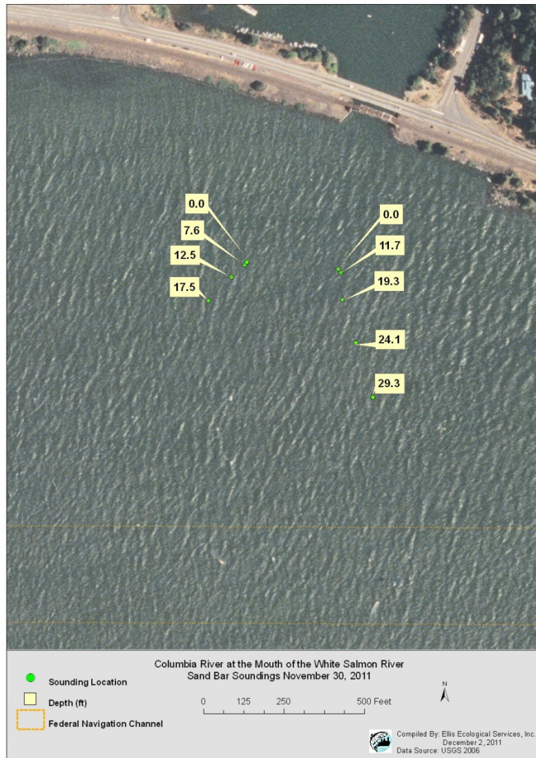
Photo 3. Depth to sediment surface measurements taken on November 30, 2011. Columbia River at the mouth of the White Salmon River. Note: photography is from an earlier date.
