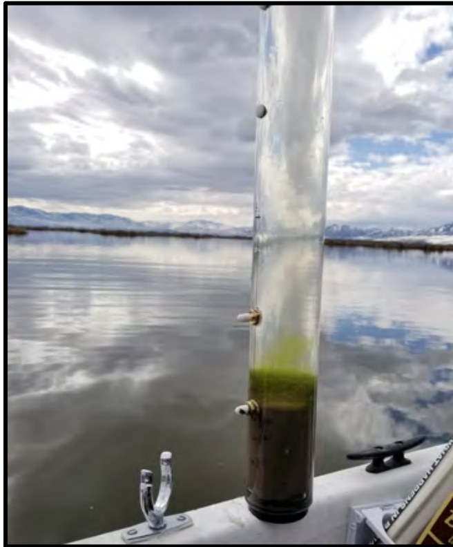
PHOTO 4-1 EXAMPLE OF INTEGRATED COLUMN SAMPLE FOR THE SEDIMENT STUDY TAKEN FROM CUTLER IN MARCH 2020
