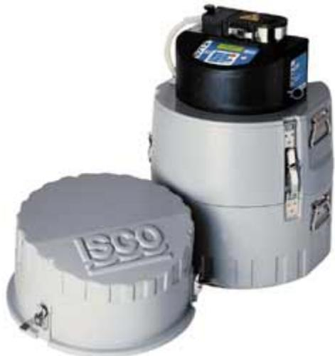
The autosamplers can be programmed to automatically collect specific volumes of samples at specific time intervals. The autosamplers use a peristaltic pump for sample collection, which compensates for pumping head and triggers automatic suction line rinsing following sampling to prevent cross contamination. Each sampling cycle includes
