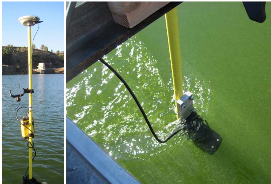
.Figure 4. Trimble GeoXT and Hydrolite-TM boat setup in Iron Gate Reservoir.
