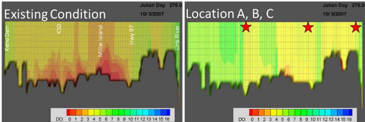
Figure 12. DO concentrations (mg/L) for existing conditions and sparging at Locations A, B, and C on October 3, 2007.
