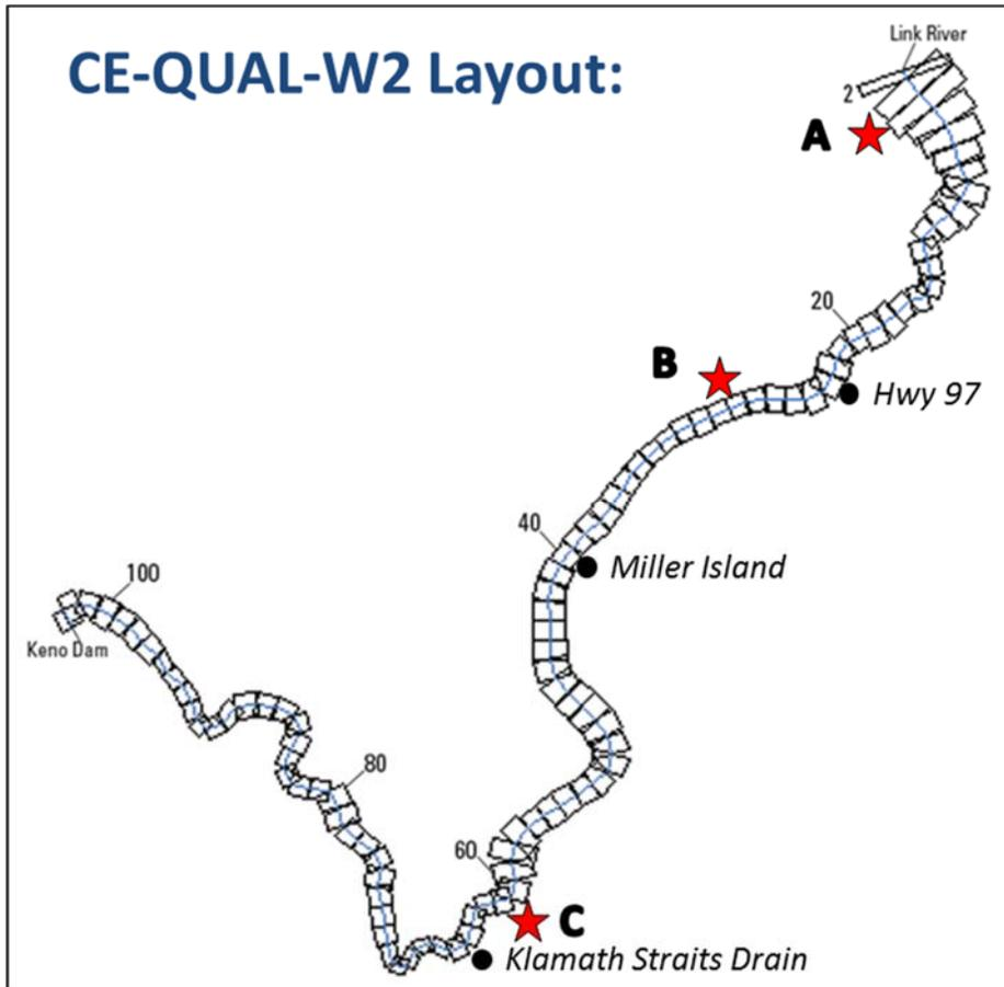
Figure 2. Keno reservoir CE-QUAL-W2 model grid and potential locations (A, B, and C) for oxygenation facilities used in this analysis.
