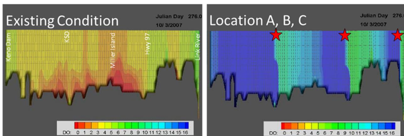
Figure 11. DO concentrations (mg/L) for existing conditions and assumed Alternative 1 side-stream oxygenation at Locations A, B, and C on October 3, 2007.
