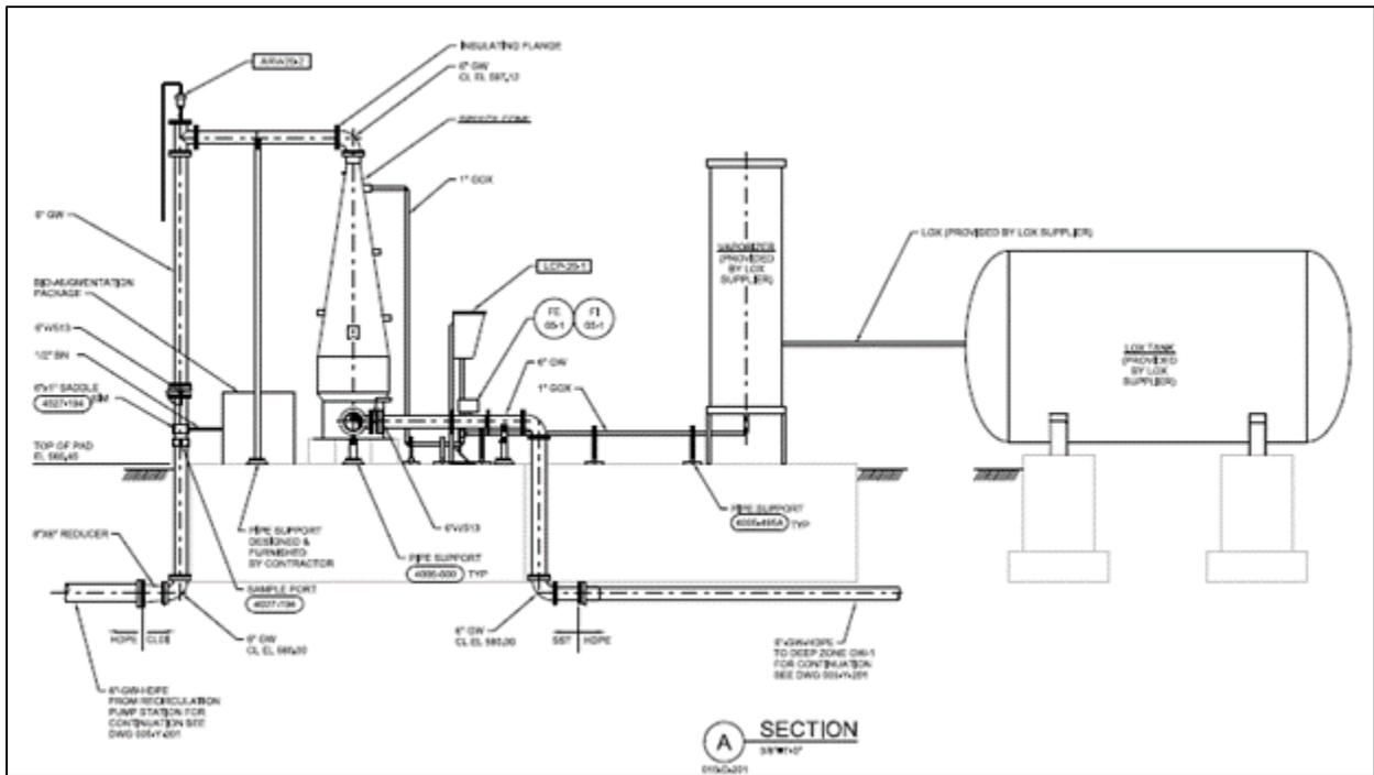
Figure 7. Example construction drawing of a Speece cone for above-water installation. Source: CH2M Unpublished Data.
