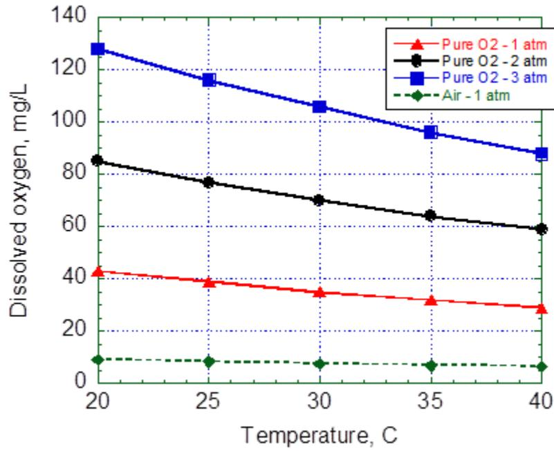
Figure 5. Dissolved oxygen saturation concentrations in air by temperature and pure oxygen by pressure and temperature.
