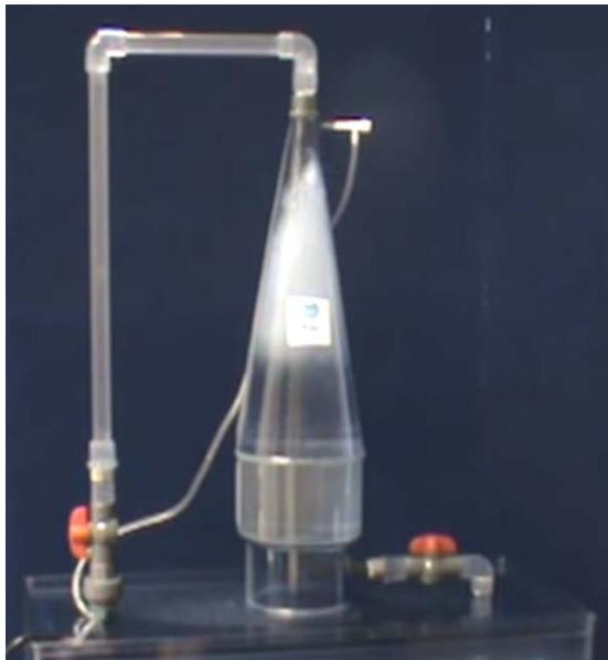
Figure 4. Small scale model of a downflow side-stream oxygenation bubble contactor (Speece cone) with schematic flows and in-cone bubble water velocities. Source: Image Eco2 Technologies.
