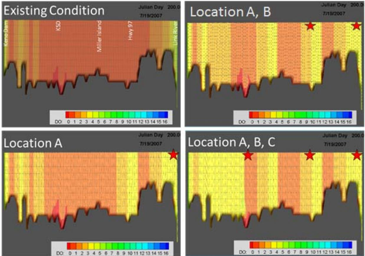
Figure 9. Model simulations of existing conditions and oxygenation via sparging at Locations A, B, and C (showing example model simulation output for July 19, 2007 at midnight).
