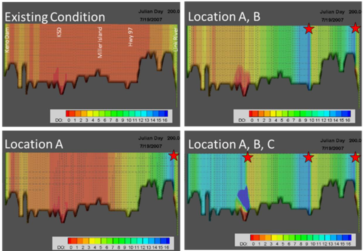
Figure 10. Model simulations of existing conditions and side-stream oxygenation at Locations A, B, and C (showing example model simulation output for July 19, 2007 at midnight). Note that the zone of supersaturation is small at locations A and B because of BOD. At location C, BOD has been sufficiently consumed to allow for a larger plume of supersaturated water.
