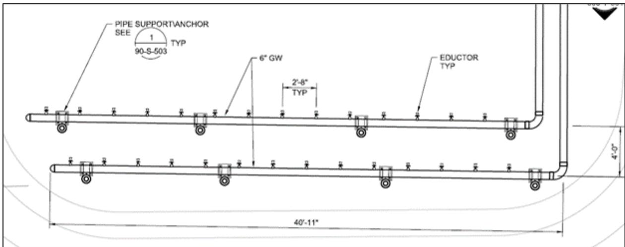
Figure 8. Example construction drawing of an eductor diffuser for injection of DO supersaturated water. Source: CH2M Unpublished Data.
