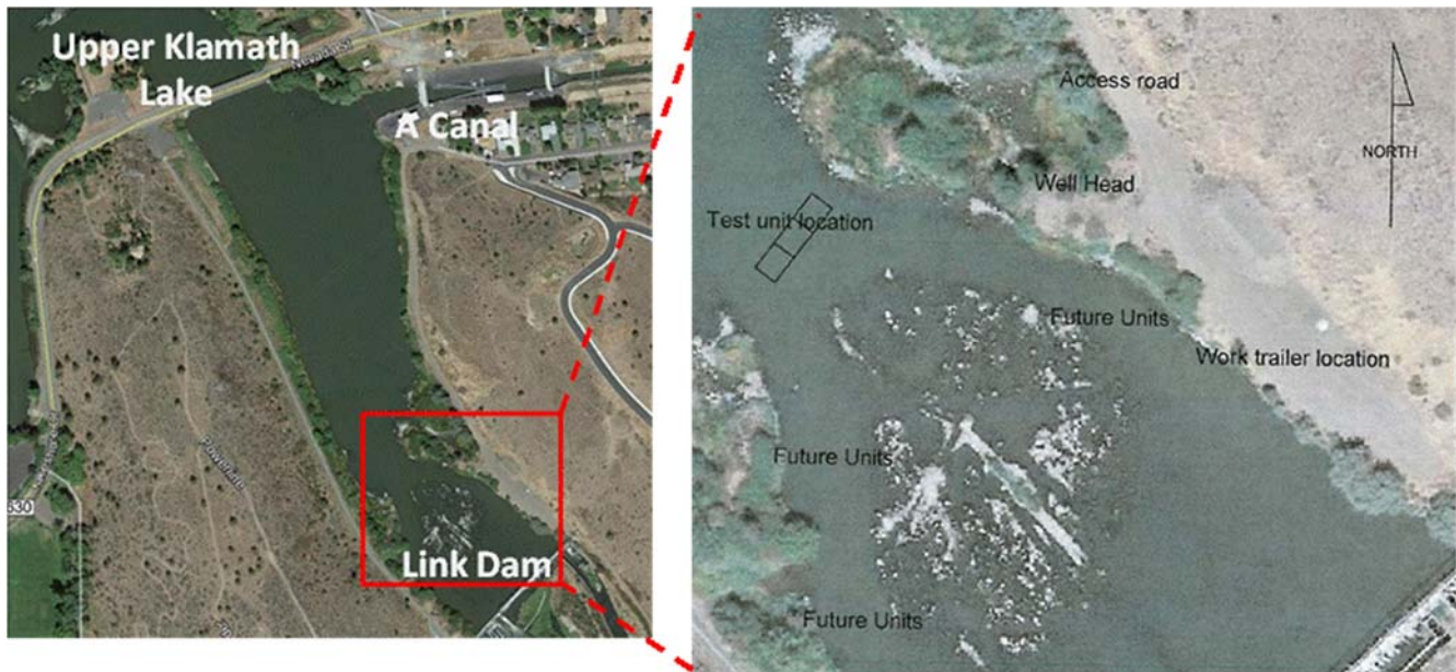
Figure 1. Proposed Link River Algae Removal Demonstration Project facilities location and layout.
