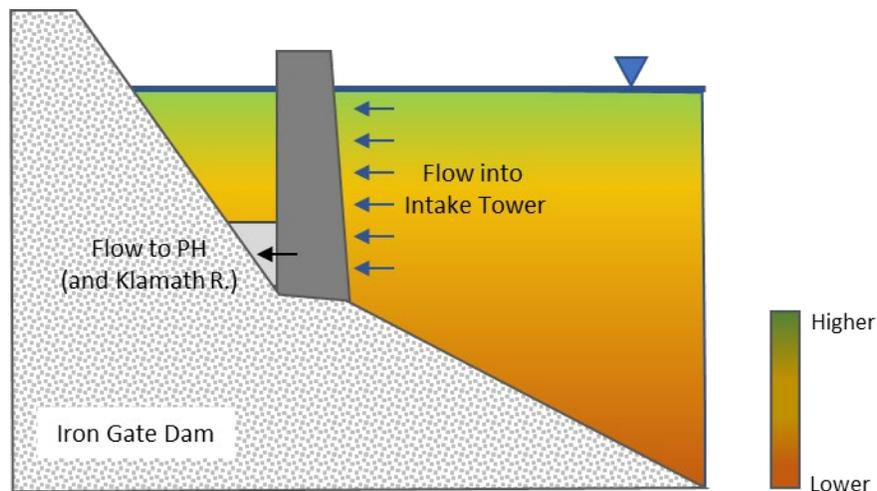
**Figure 4-4. Conceptual diagram of vertical cyanobacteria distribution showing Iron Gate Dam intake tower region with flow entering from full depth (no curtain): summertime.**
