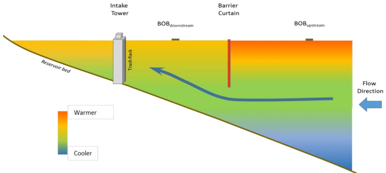
**Figure 2-8. Conceptual profile view of thermal conditions in Iron Gate Reservoir showing the location of the barrier curtain, upstream of the curtain and downstream of the curtain Basic Observation Buoys (BOBs), and intake tower.**
