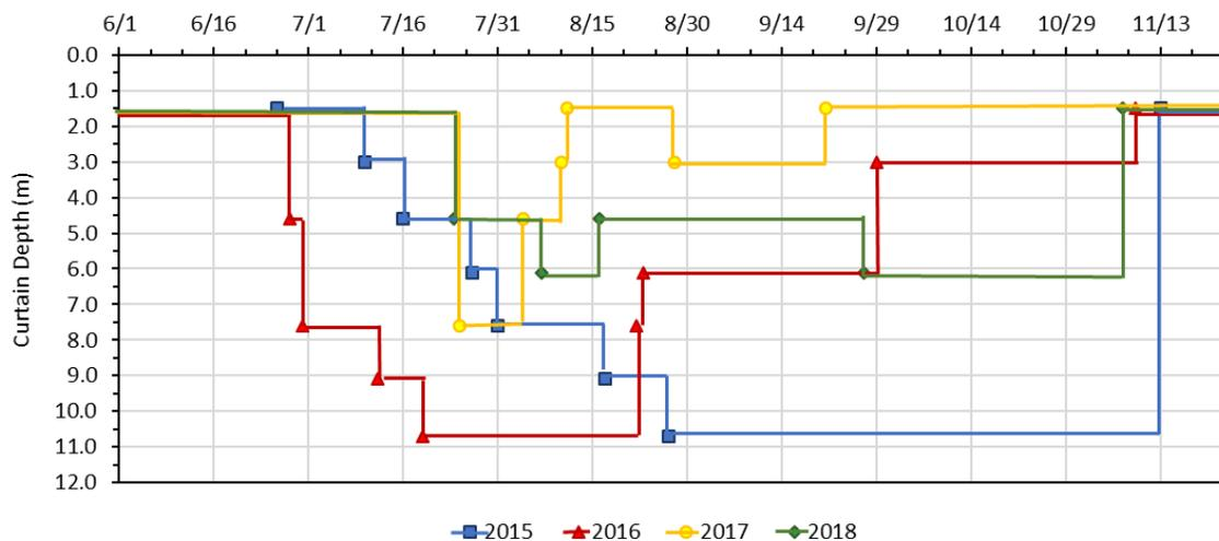
**Figure 5-1. 2015-2018 Deployment depths in meters (m) for the Intake Barrier Curtain in Iron Gate Reservoir.**
