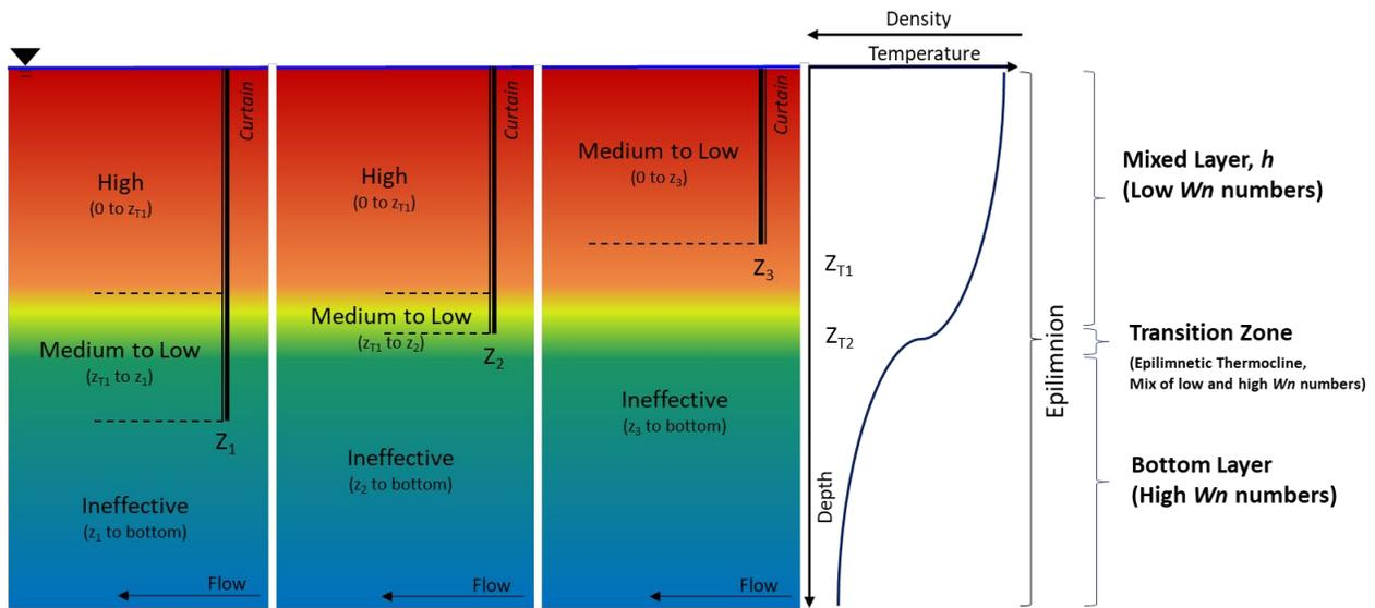
**Figure 4-2. Curtain deployed conditions and potential curtain effectiveness (Condition 1 – left panel, Condition 2 – middle panel, Condition 3 – Right panel).**
