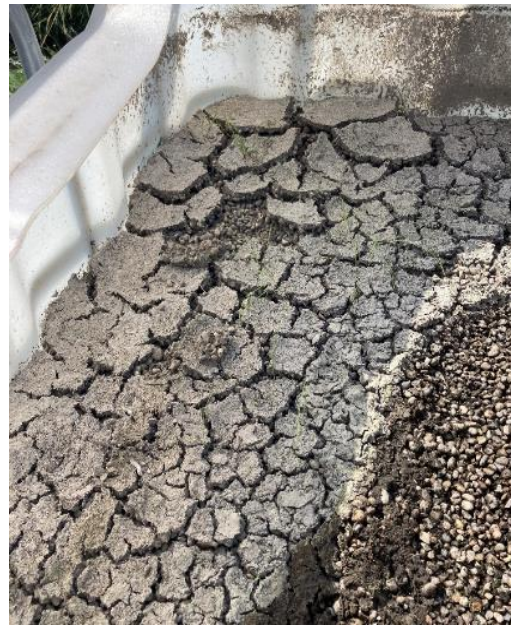
Figure 9. (left) Impervious mud formation hindering flow rates through the biochar media (7/28/21) (right) Sediment-mud layer after drying down prior to pea gravel replacement (8/17/21)
