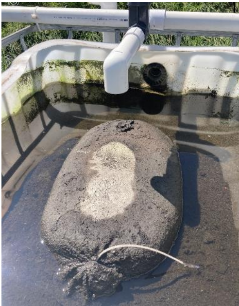
Figure 9. (left) Impervious mud formation hindering flow rates through the biochar media (7/28/21) (right) Sediment-mud layer after drying down prior to pea gravel replacement (8/17/21)
