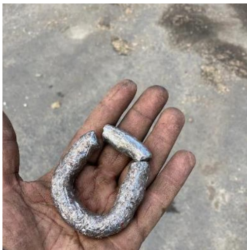
Figure 5. Metal choker chain fragment found in the wood fiber
