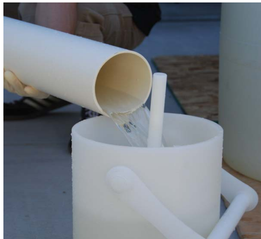
Figure A-2. Pouring water sample into the churn splitter.
