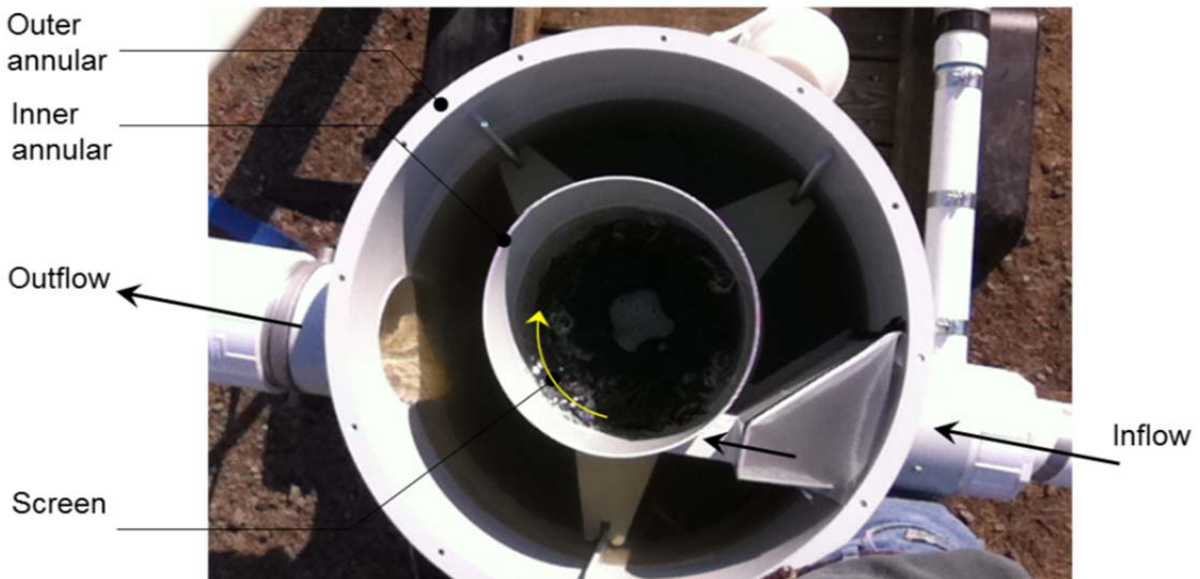
Figure 5. Top View of Prototype Separator with Arrows Indicating the Direction of Flow
