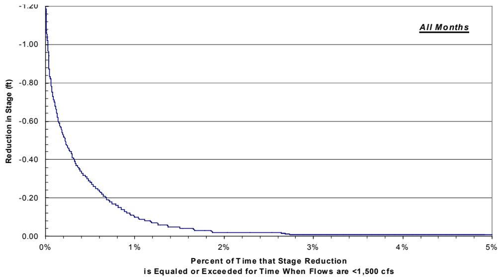
Figure 6.7-3. Klamath River at Keno: hourly reduction for flows less than 1,500 cfs, water years 1990 through 2001.
