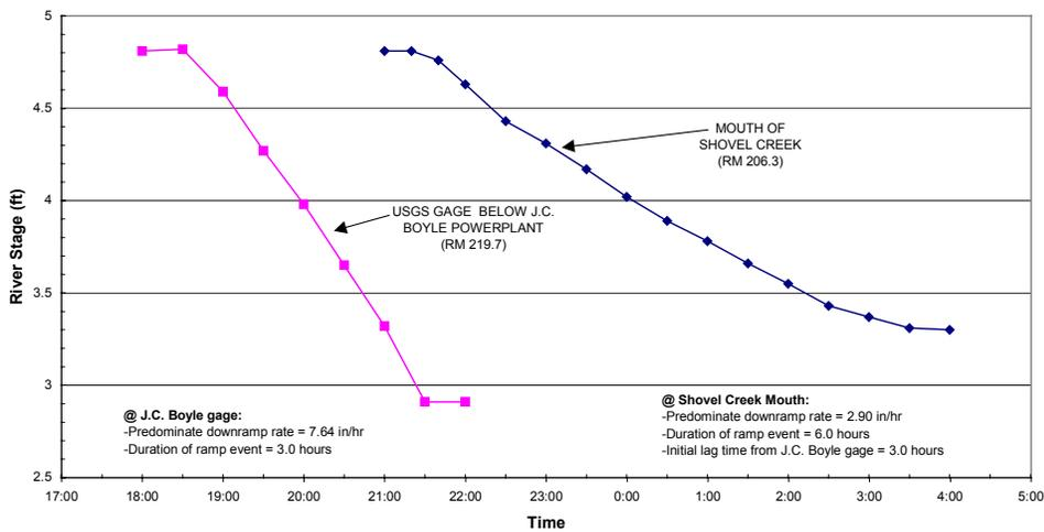
Figure 6.7-18. Klamath River stage reduction comparison between J.C. Boyle gauge and surveyed data at mouth of Shovel Creek—August 20, 2003. (Distance = 13.4 miles. Flow reduced from 1,710 cfs to 350 cfs.)
