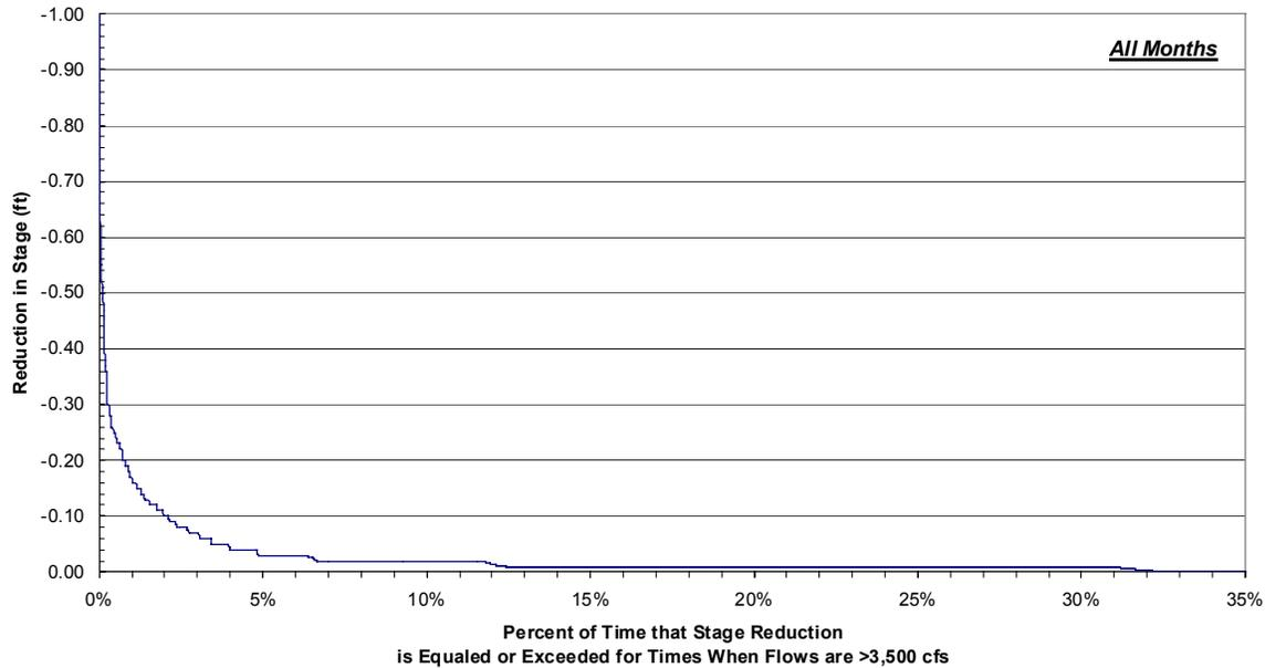
Figure 6.7-5. Klamath River at J.C. Boyle bypass: hourly reduction of stage for flow greater than 3,500 cfs, water years 1991 through 2001.
