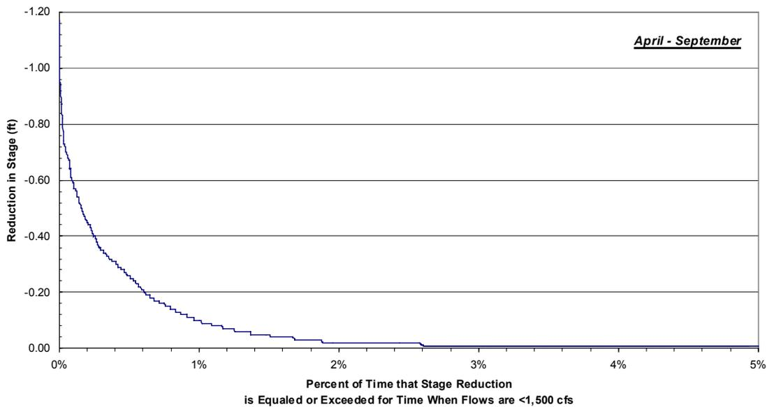
Figure 6.7-4. Klamath River at Keno: hourly reduction of state for flows less than 1,500 cfs, April through September 1990 through 2001.
