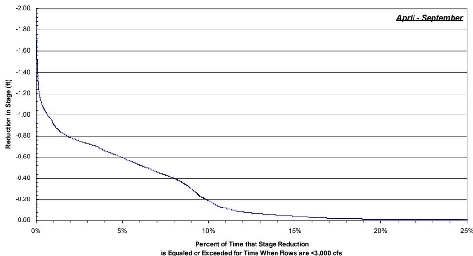
Figure 6.7-7. Klamath River at J.C. Boyle peaking: hourly reduction of stage for flow less than 3,000 cfs, April through September 1991 through 2001 (excluding 1996).
