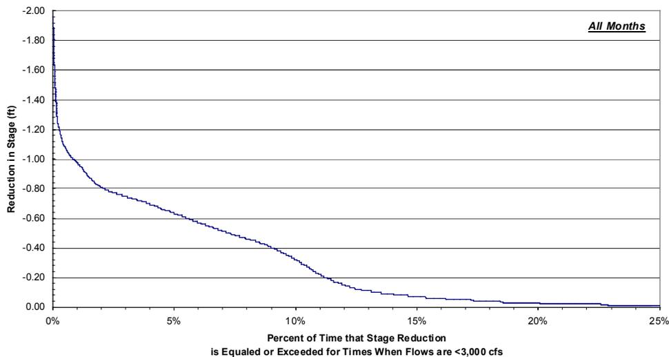
Figure 6.7-6. Klamath River at J.C. Boyle peaking: hourly reduction of stage for flow less than 3,000 cfs, water years 1991 through 2001.
