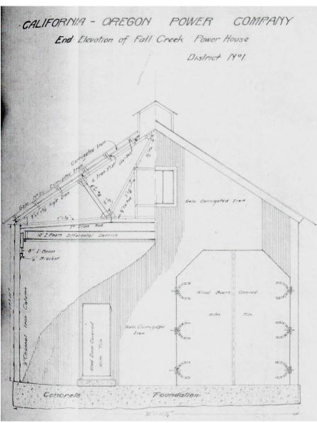
Figure 27: Cross-Section of the Fall Creek Powerhouse, 1915 (Source: PacifiCorp Archive, Box 43959)
