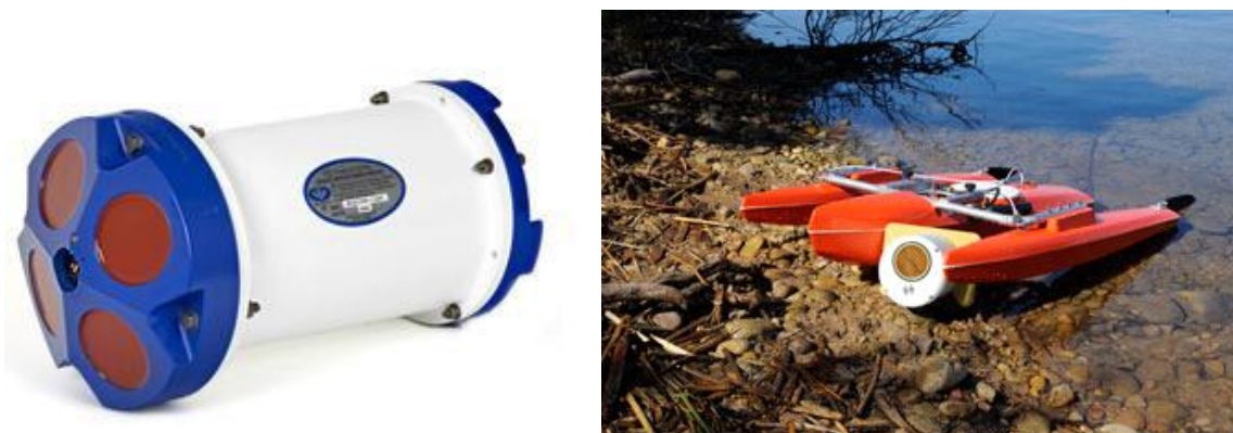
Figure 3. Workhouse Sentinel acoustic Doppler current profiler (ADCP) by Teledyne RD Instruments, and cataraft used to deploy ADCP in reservoir (source: Teledyne Technologies (2007b)).
