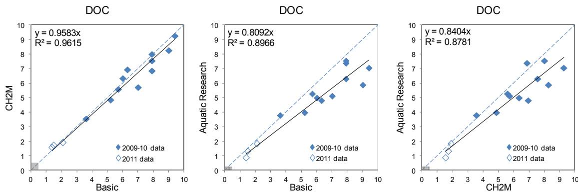
**Figure D-12.** KHSAs inter-laboratory plots from 2009-2011 for Dissolved Organic Carbon. Units in milligrams per liter (mg/l). Grey region in lower left corner of each plot depicts concentrations below the reporting limits for respective laboratories in 2011.
