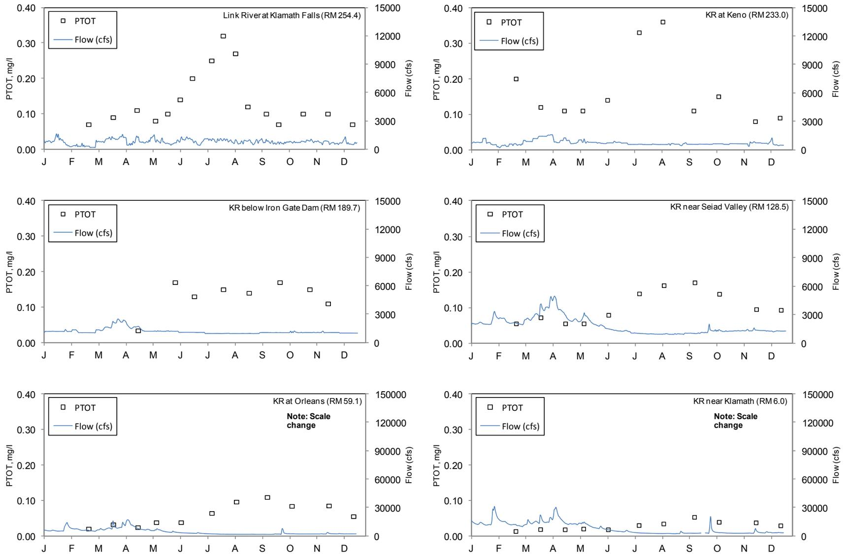
**Figure 16. Total phosphorus (PTOT) and daily flow at USGS flow gage locations for the mainstem Klamath and Link Rivers. Note the scale change for the secondary y-axis at Orleans and Klamath. (2013)**
