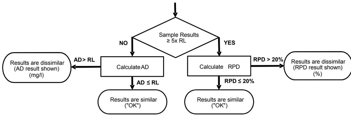
**Figure D-2. Flow diagram of the comparison process. RPD = relative percent difference. RL = reporting limit. AD = absolute difference.**
