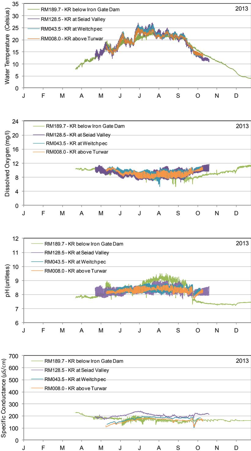
**Figure 11. Water temperature, dissolved oxygen, pH, specific conductance data (2013) for the lower Klamath River at Klamath River below Iron Gate Dam, Klamath River near Seiad Valley, Klamath River at Weitchpec, and Klamath River above Turwar. Continuous data was collected using data sondes.**
