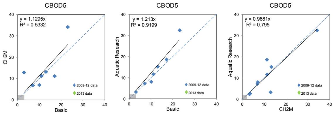
**Figure E-11. KHSA inter-laboratory plots from 2009-2013 for Carbonaceous Biological Oxygen Demand. Units in milligrams per liter (mg/l). Grey region in lower corner shows concentrations below the RL for the respective laboratories in 2013.**
