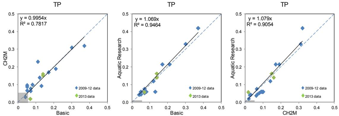
**Figure E-4. KHSa inter-laboratory plots from 2009-2013 for Total Phosphorus. Units in milligrams per liter (mg/l). Grey region in lower corner shows concentrations below the RL for the respective laboratories in 2013.**
