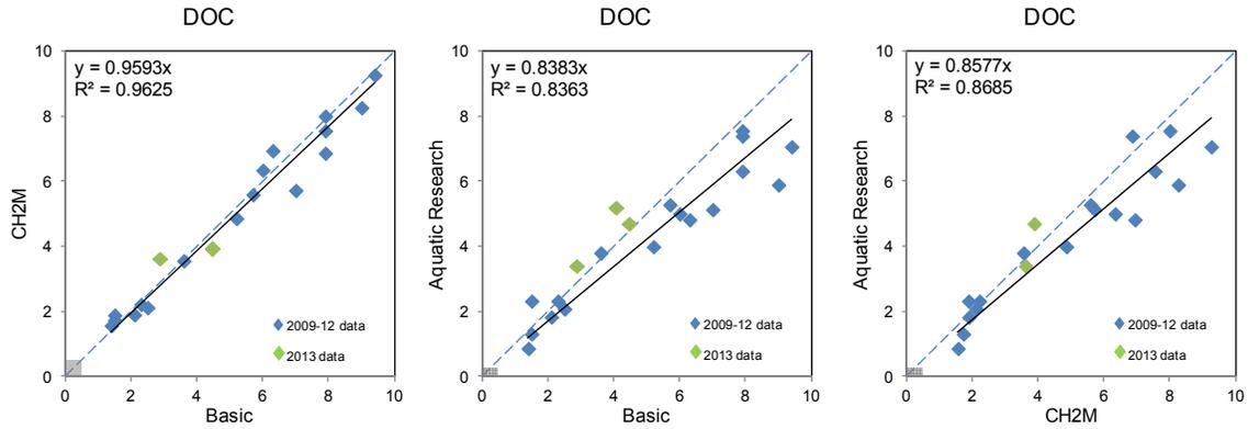
**Figure E-10. KHSA inter-laboratory plots from 2009-2013 for Dissolved Organic Carbon. Units in milligrams per liter (mg/l). Grey region in lower corner shows concentrations below the RL for the respective laboratories in 2013.**
