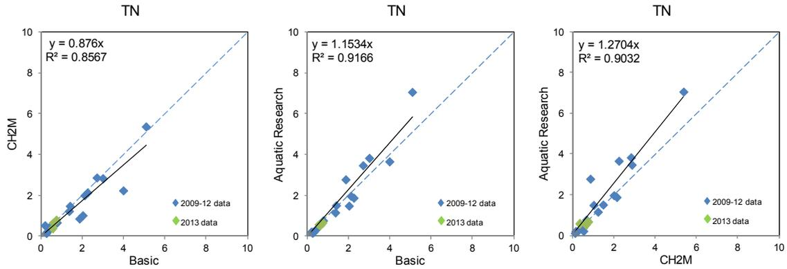
**Figure E-7. KHSA inter-laboratory plots from 2009-2013 for Total Nitrogen. Units in milligrams per liter (mg/l). Grey region in lower corner shows concentrations below the RL for the respective laboratories in 2013.**
