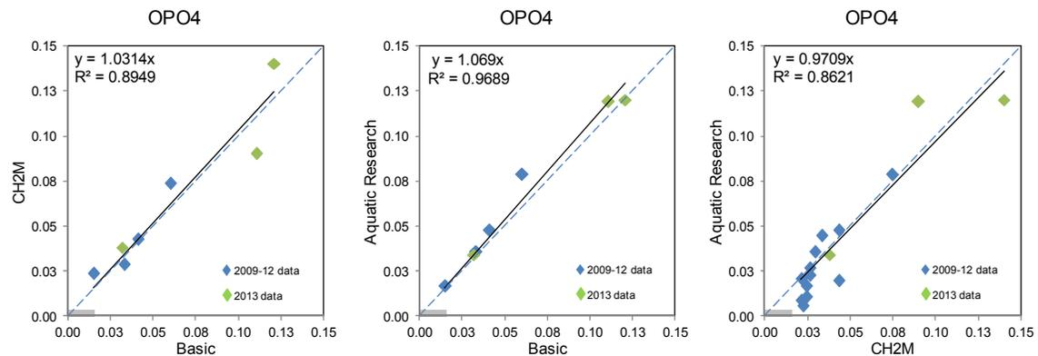
**Figure E-5. KHSa inter-laboratory plots from 2009-2013 for Orthophosphate. Units in milligrams per liter (mg/l). Grey region in lower corner shows concentrations below the RL for the respective laboratories in 2013.**
