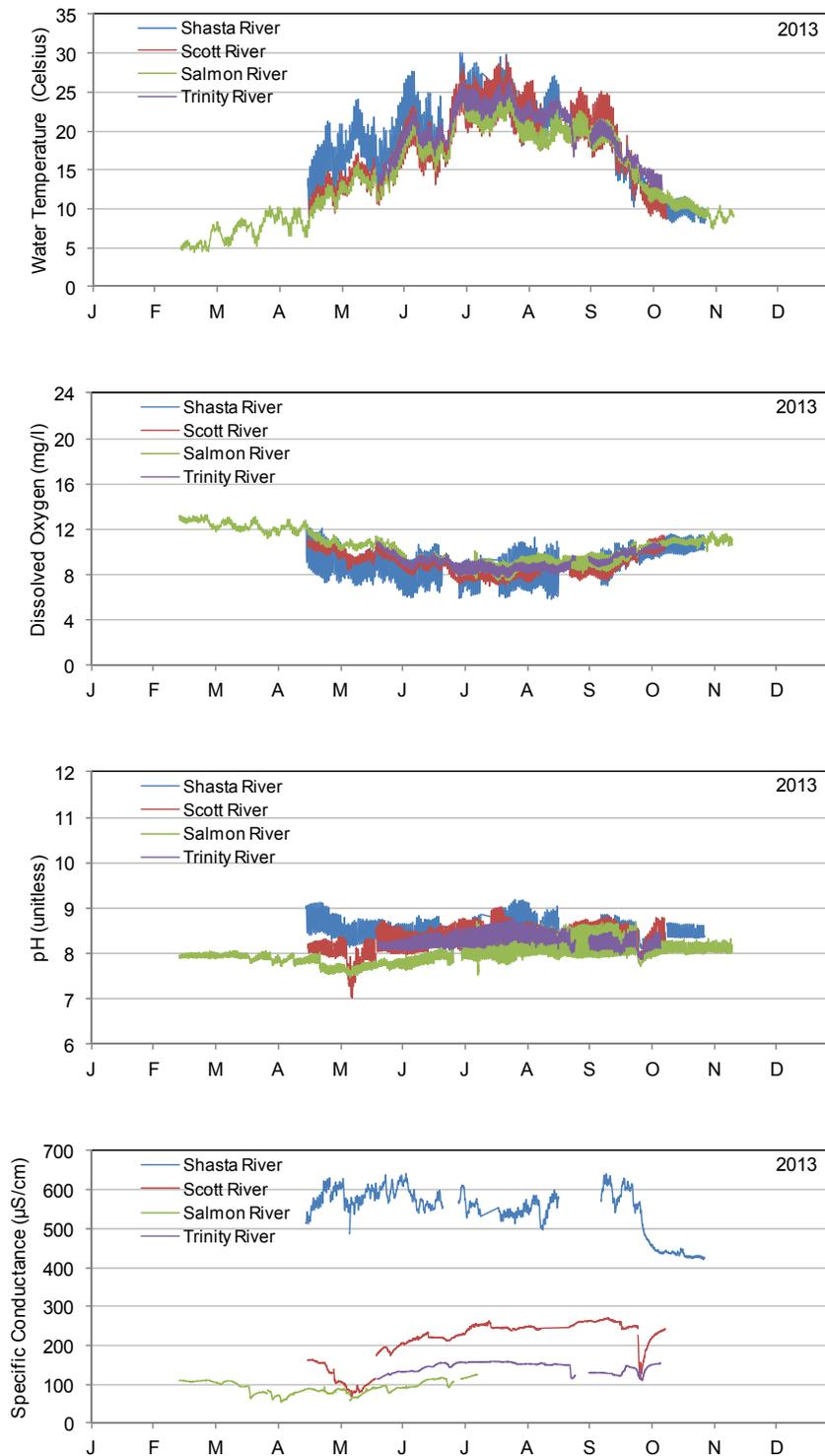
**Figure 9. Water temperature, dissolved oxygen, pH, specific conductance data (2013) for the Shasta River, Scott River, Salmon River, and Trinity River. Continuous data was collected using data sondes.**
