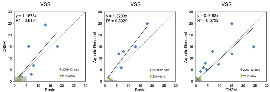
**Figure E-3. KHSA inter-laboratory plots from 2009-2013 for Volatile Suspended Solids. Units in milligrams per liter (mg/l). Grey region in lower corner shows concentrations below the RL for the respective laboratories in 2013.**
