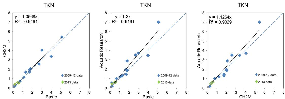
**Figure E-6. KHSa inter-laboratory plots from 2009-2013 for Total Kjeldahl Nitrogen. Units in milligrams per liter (mg/l). Grey region in lower corner shows concentrations below the RL for the respective laboratories in 2013.**
