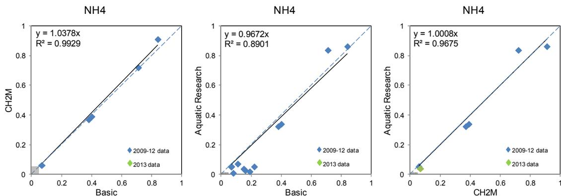
**Figure E-8. KHSA inter-laboratory plots from 2009-2013 for Ammonia. Units in milligrams per liter (mg/l). Grey region in lower corner shows concentrations below the RL for the respective laboratories in 2013.**
