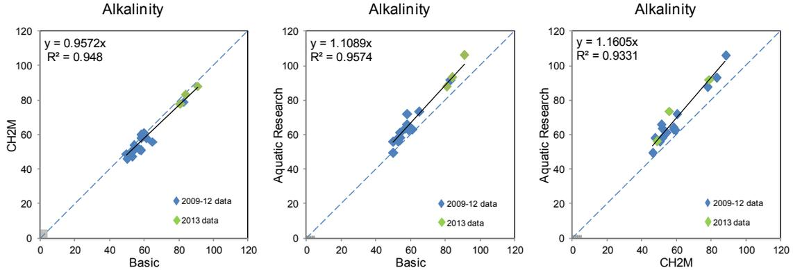
**Figure E-1. KHSA inter-laboratory plots from 2009-2013 for Alkalinity. Units in milligrams per liter (mg/l). Grey region in lower corner shows concentrations below the RL for the respective laboratories in 2013.**
