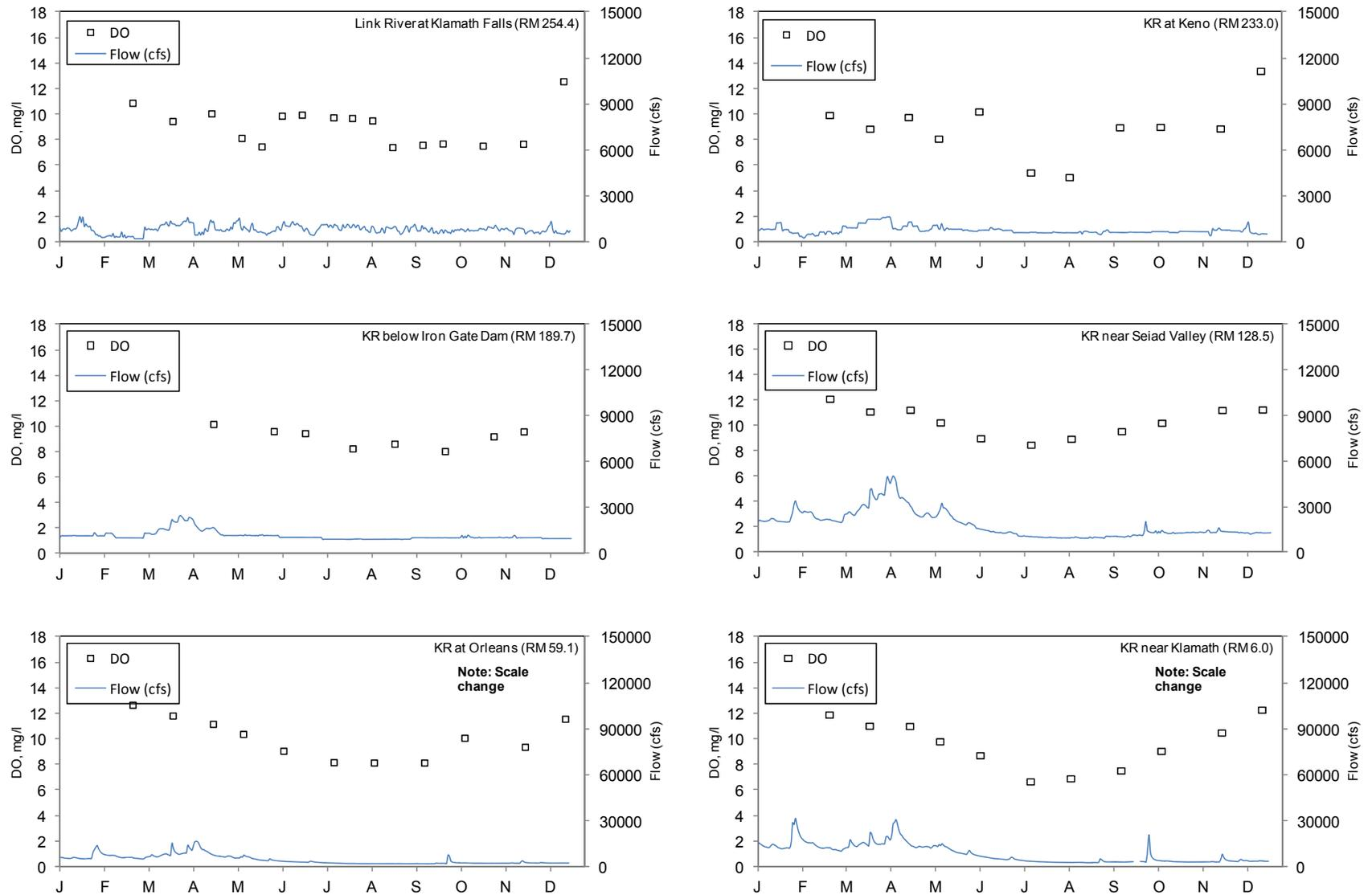
Figure 13. Dissolved oxygen (DO) and daily flow at USGS flow gage locations for the mainstem Klamath and Link Rivers. Note the scale change for the secondary y-axis at Orleans and near Klamath mouth. (2013)
