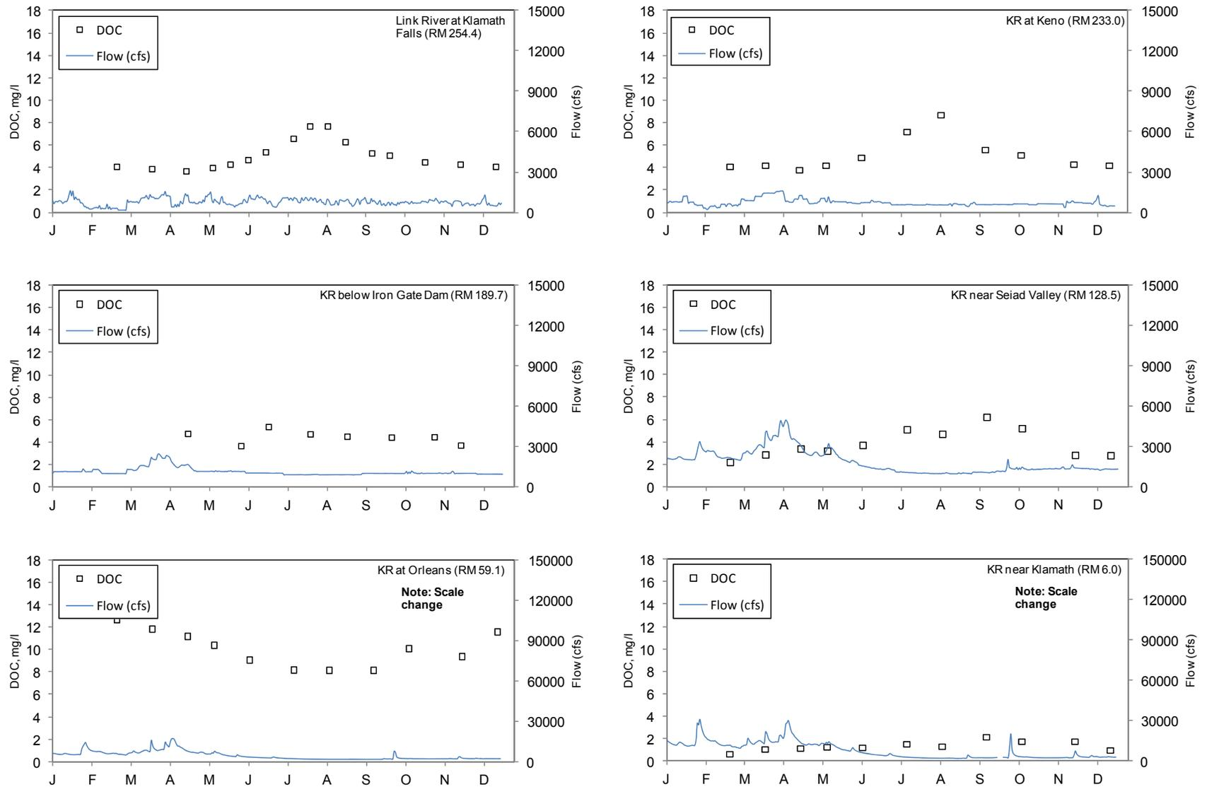
Figure 14. Dissolved organic carbon (DOC) and daily flow at USGS flow gage locations for the mainstem Klamath and Link Rivers. Note the scale change for the secondary y-axis at Orleans and near Klamath mouth. (2013)
