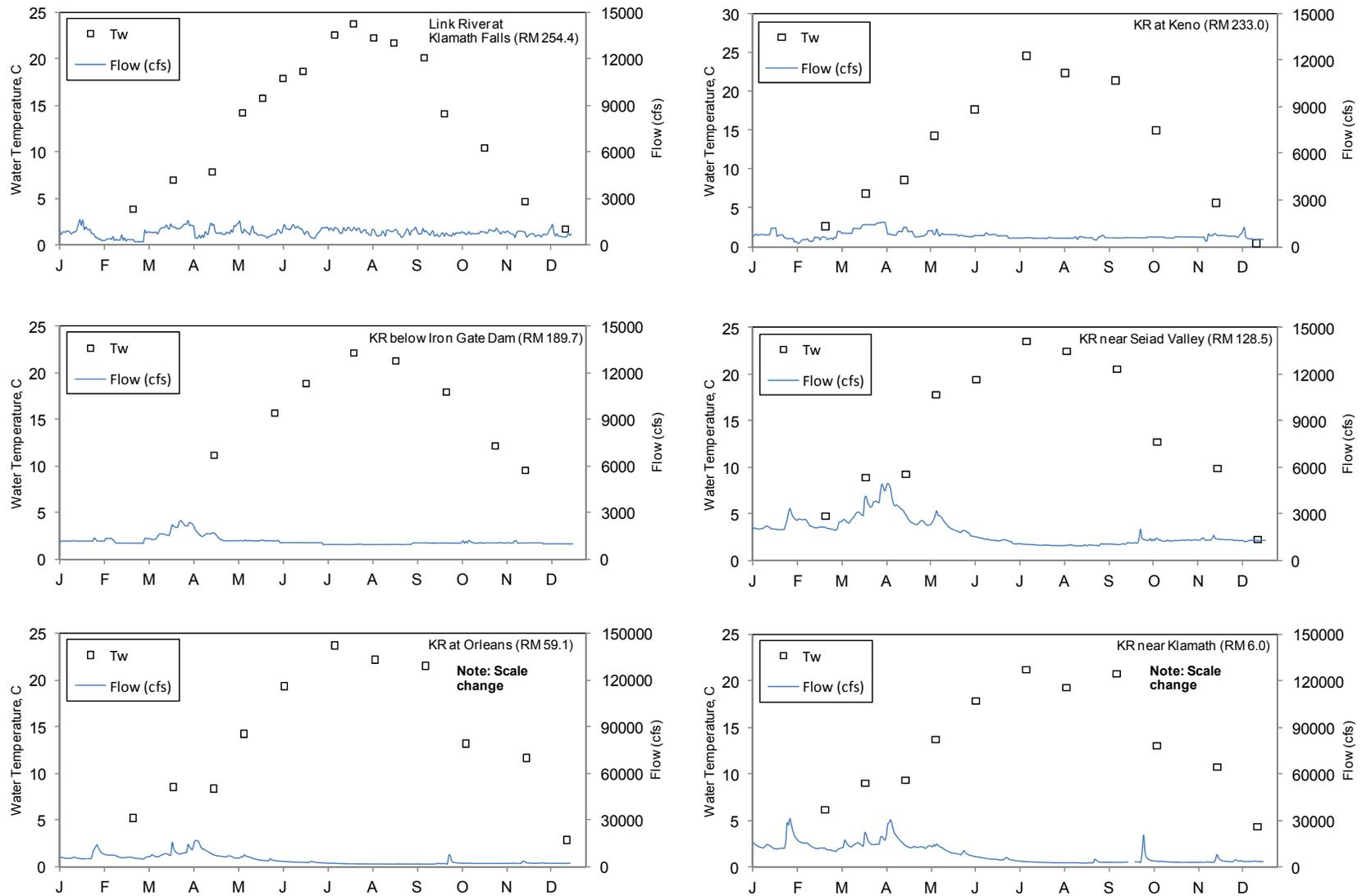
**Figure 12. Water temperature ( $T_w$ ) and daily flow at USGS flow gage locations for the mainstem Klamath and Link Rivers. Note the scale change for the secondary y-axis at Orleans and near Klamath mouth. (2013)**
