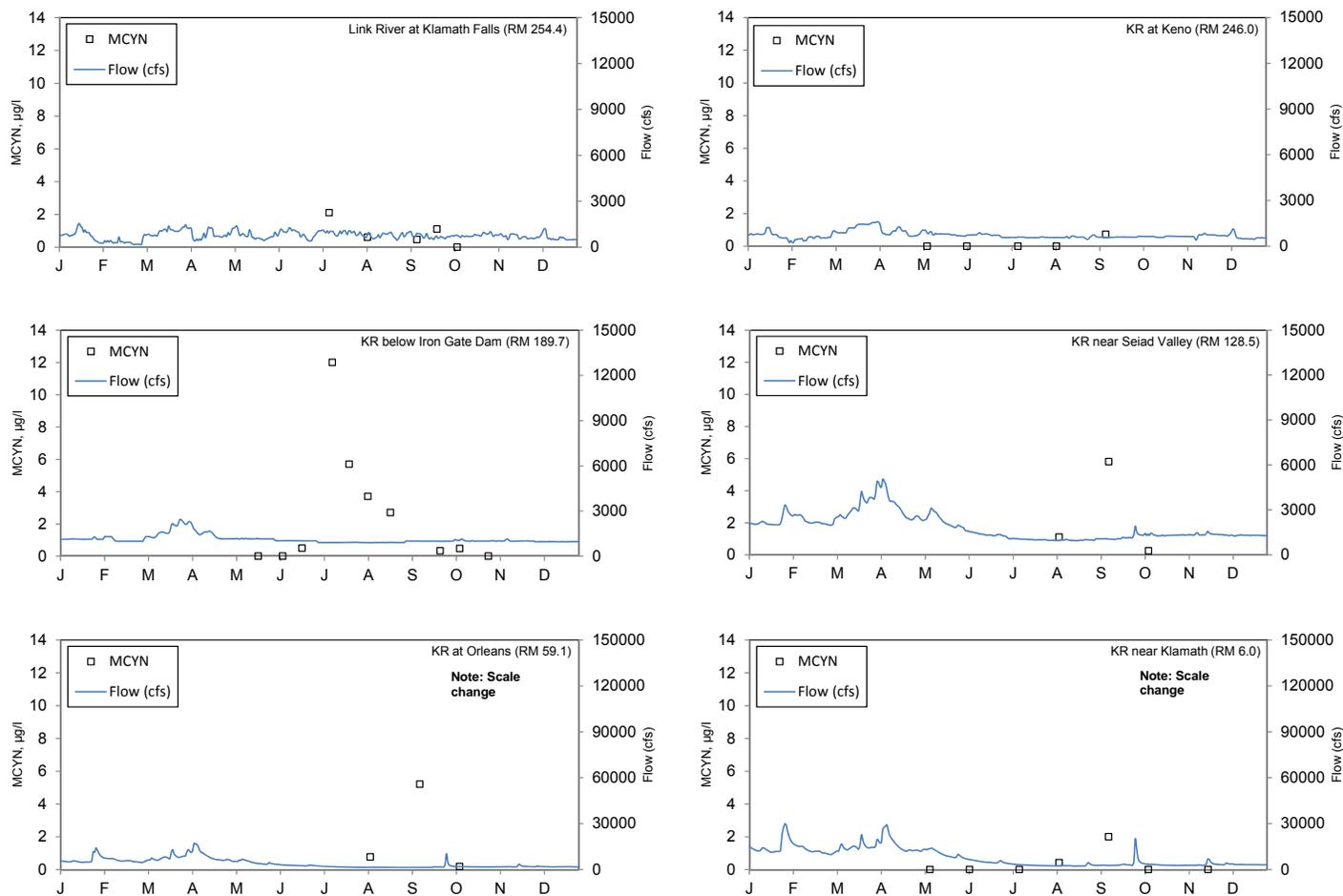
**Figure 17. 2013 microcystin (MCYN) and daily flow at USGS flow gage locations for the mainstem Klamath and Link Rivers. Only surface samples are taken in consideration. Non-detect values are presented as zeros. Note the scale change for the secondary y-axis at Orleans and Klamath.**
