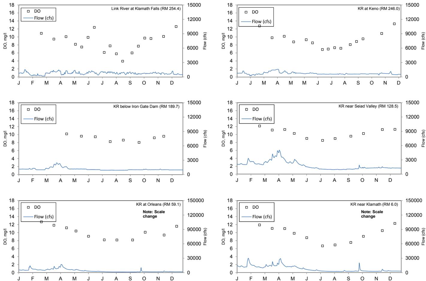
**Errata Figure13. 2013 Discrete dissolved oxygen (DO) and daily flow at USGS flow gage locations for the mainstem Klamath and Link Rivers. Note the scale change for the secondary y-axis at Orleans and near Klamath mouth.**
