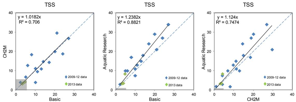
**Figure E-2. KHSA inter-laboratory plots from 2009-2013 for Total Suspended Solids. Units in milligrams per liter (mg/l). Grey region in lower corner shows concentrations below the RL for the respective laboratories in 2013.**
