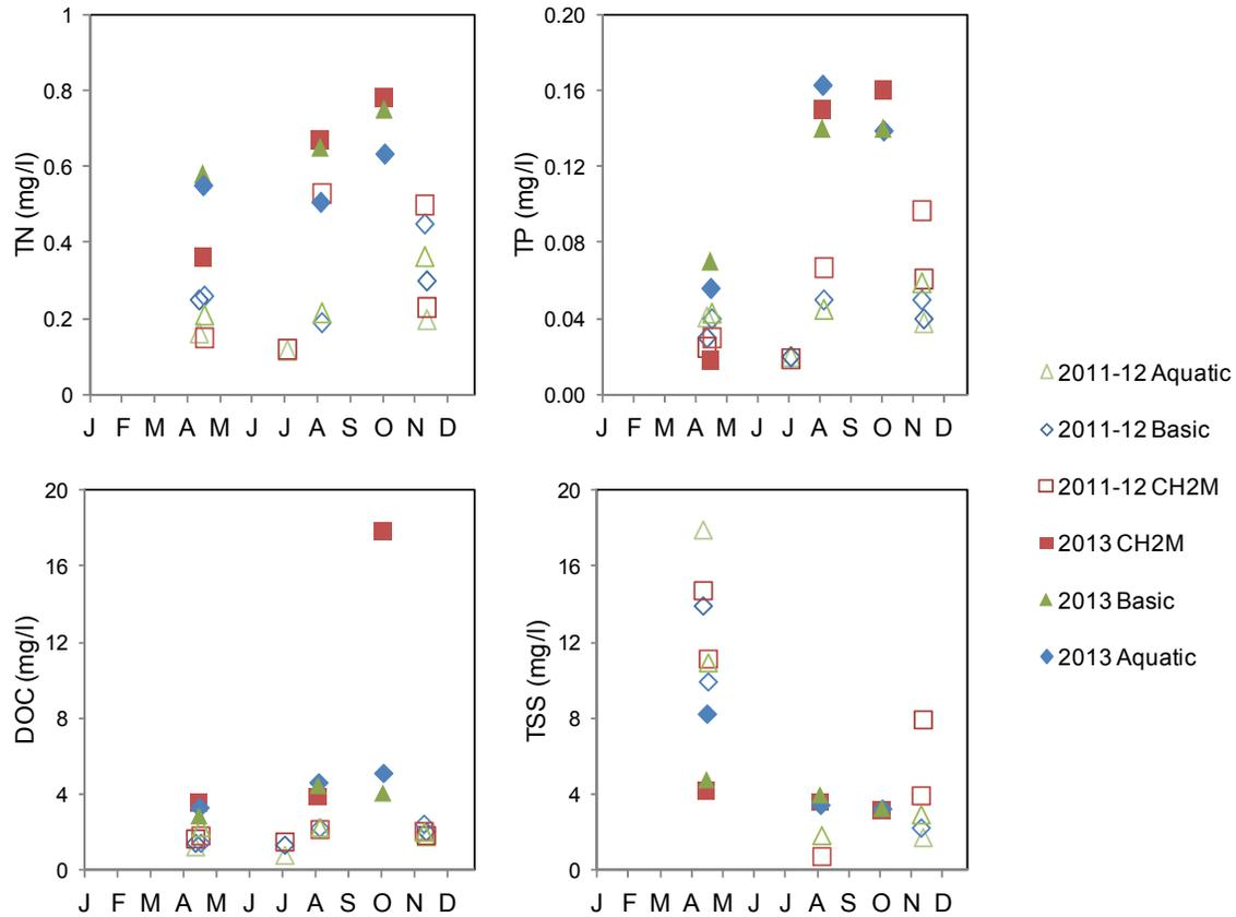
Figure D-1. 2011-2012 (outlined symbols) and 2013 (solid symbols) laboratory results for total nitrogen (TN), total phosphorus (TP), dissolved organic carbon (DOC), and total suspended solids (TSS).
