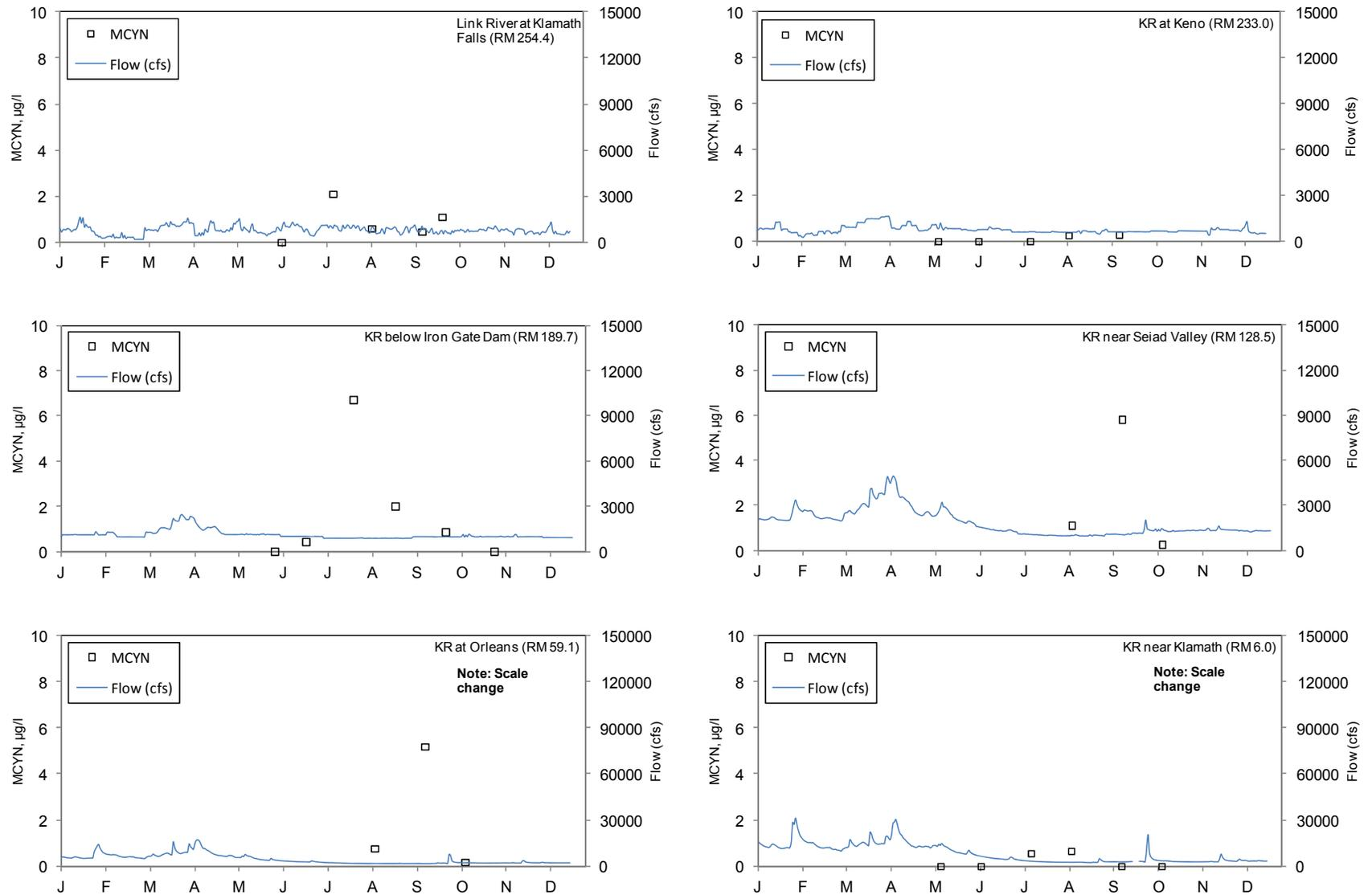
Figure 17. Microcystin (MCYN) and daily flow at USGS flow gage locations for the mainstem Klamath and Link Rivers. Only surface samples are taken in consideration. Non-detect values are presented as zeros. Note the scale change for the secondary y-axis at Orleans and Klamath. (2013)
