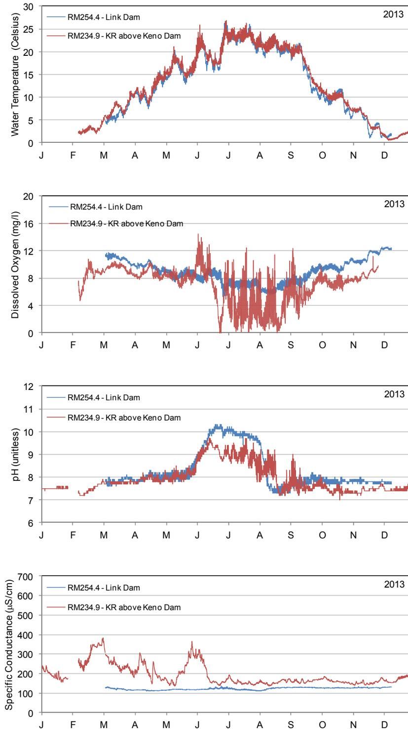
Figure 10. Water temperature, dissolved oxygen, pH, specific conductance data (2013) for the upper Klamath River at Link Dam and Klamath River above Keno Dam (near surface). Continuous data was collected using data sondes.
