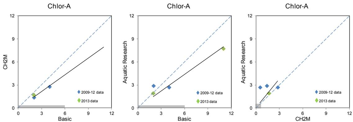
**Figure E-12. KHSA inter-laboratory plots from 2009-2013 for Chlorophyll-a. Units in micrograms per liter (µg/l). Chlorophyll-a was not collected from 2009-2011. Grey region in lower corner shows concentrations below the RL for the respective laboratories in 2013.**
