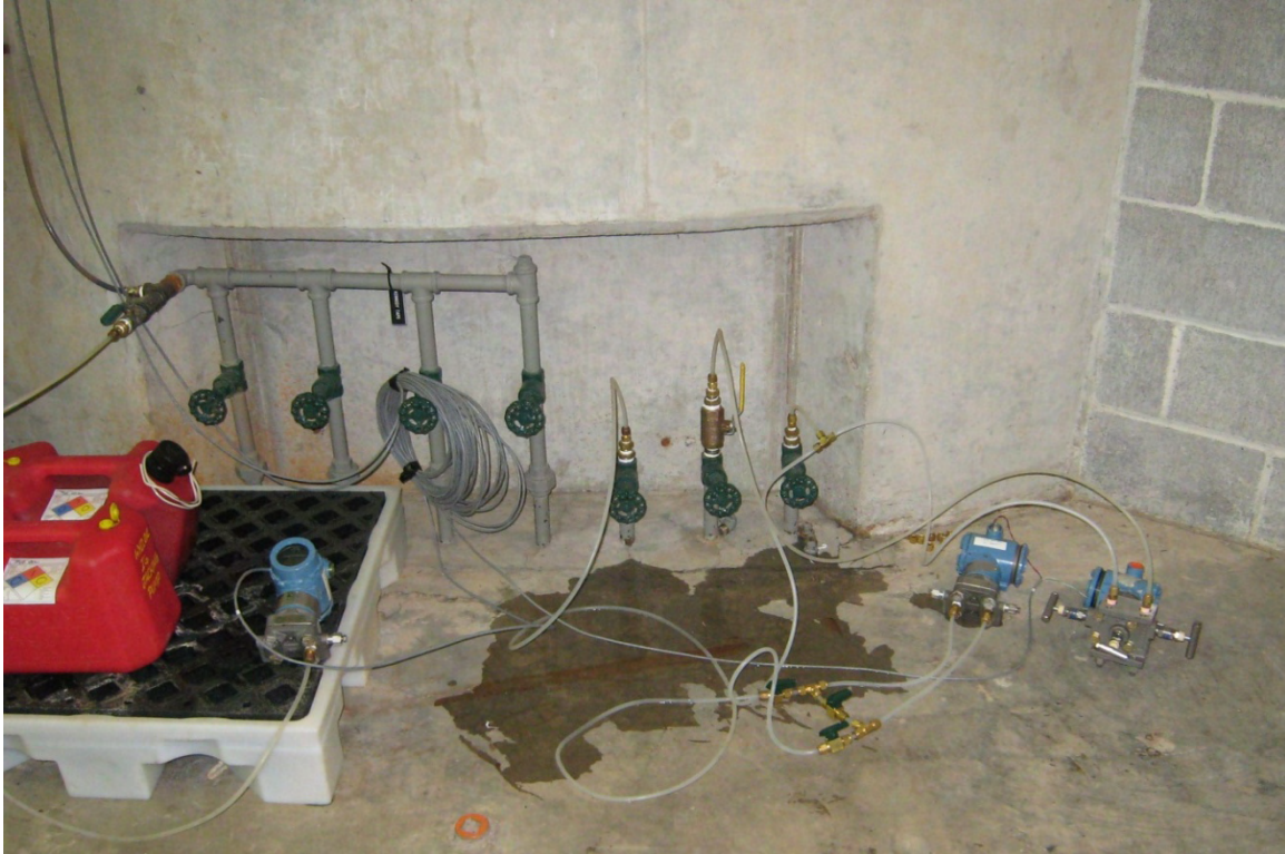
Figure 3.2: Inlet and Winter-Kennedy Pressure Cell Installation
