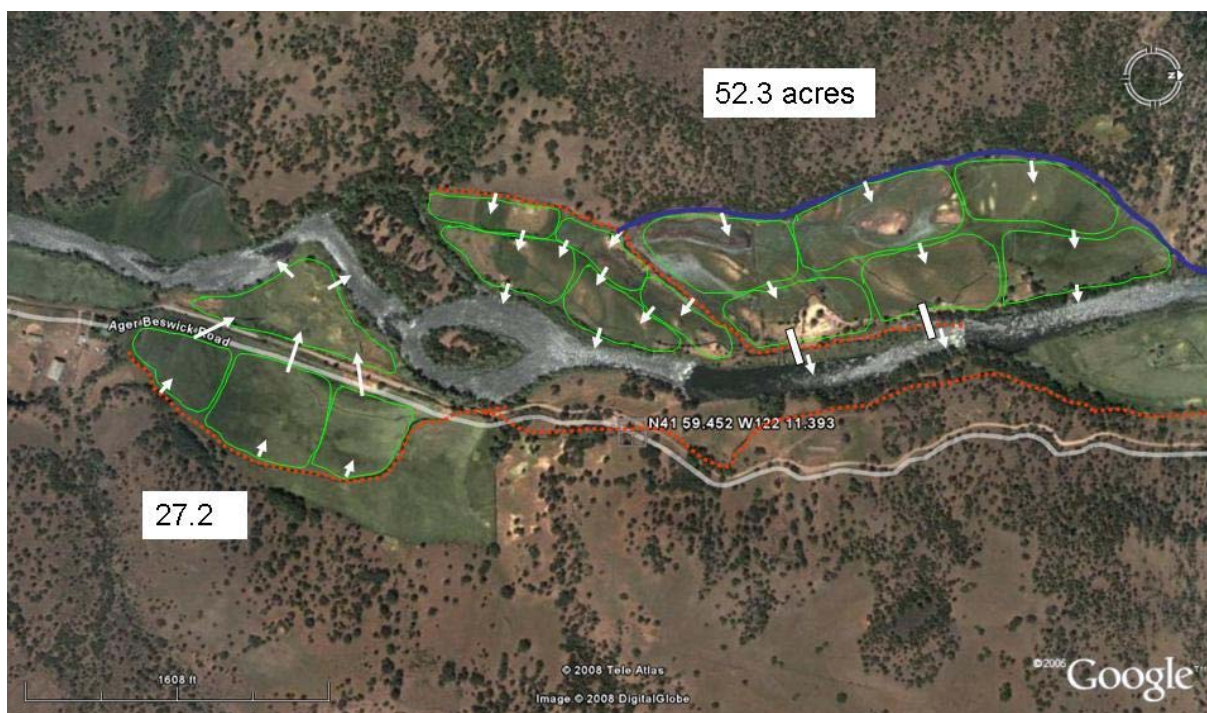
Figure 4. Conceptual layout of surface flow wetlands at Site 013 on the Klamath River upstream of Copco reservoir. As much as possible, this makes use of the pre-existing gravity fed canals (in red) and when necessary, installs new channels (in blue).
