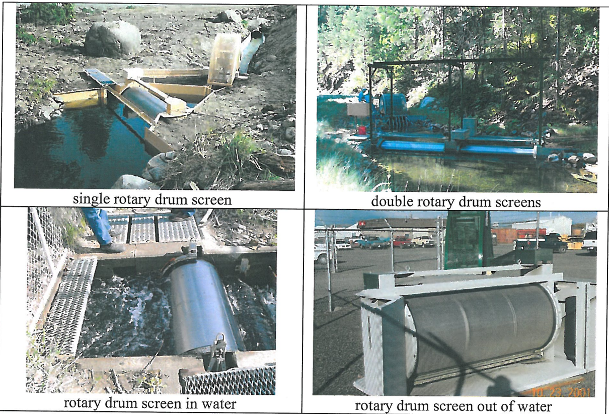
Figure 8.5. Photo examples of rotary drum screens.
