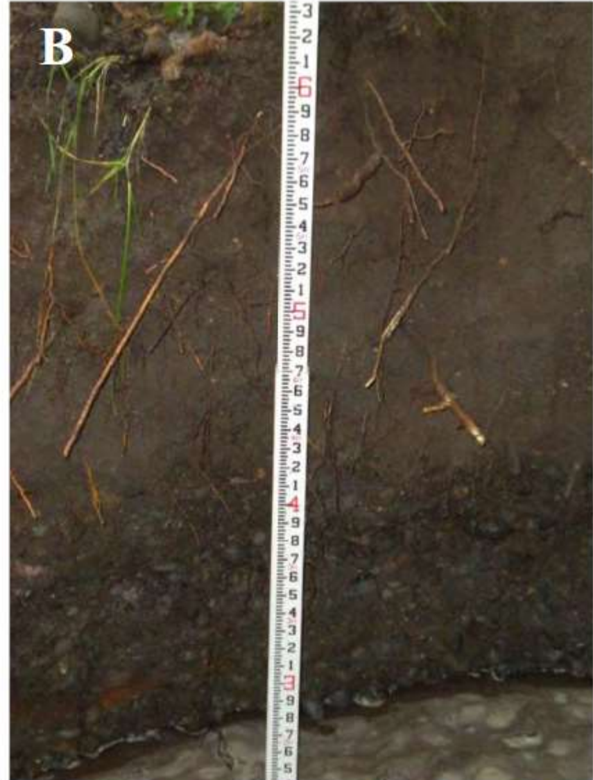
Figure 3. (A) looking upstream in the trench during the pump test. (B) The transition from soil, to sand, and finally alluvium can be seen in the wall of the trench.
