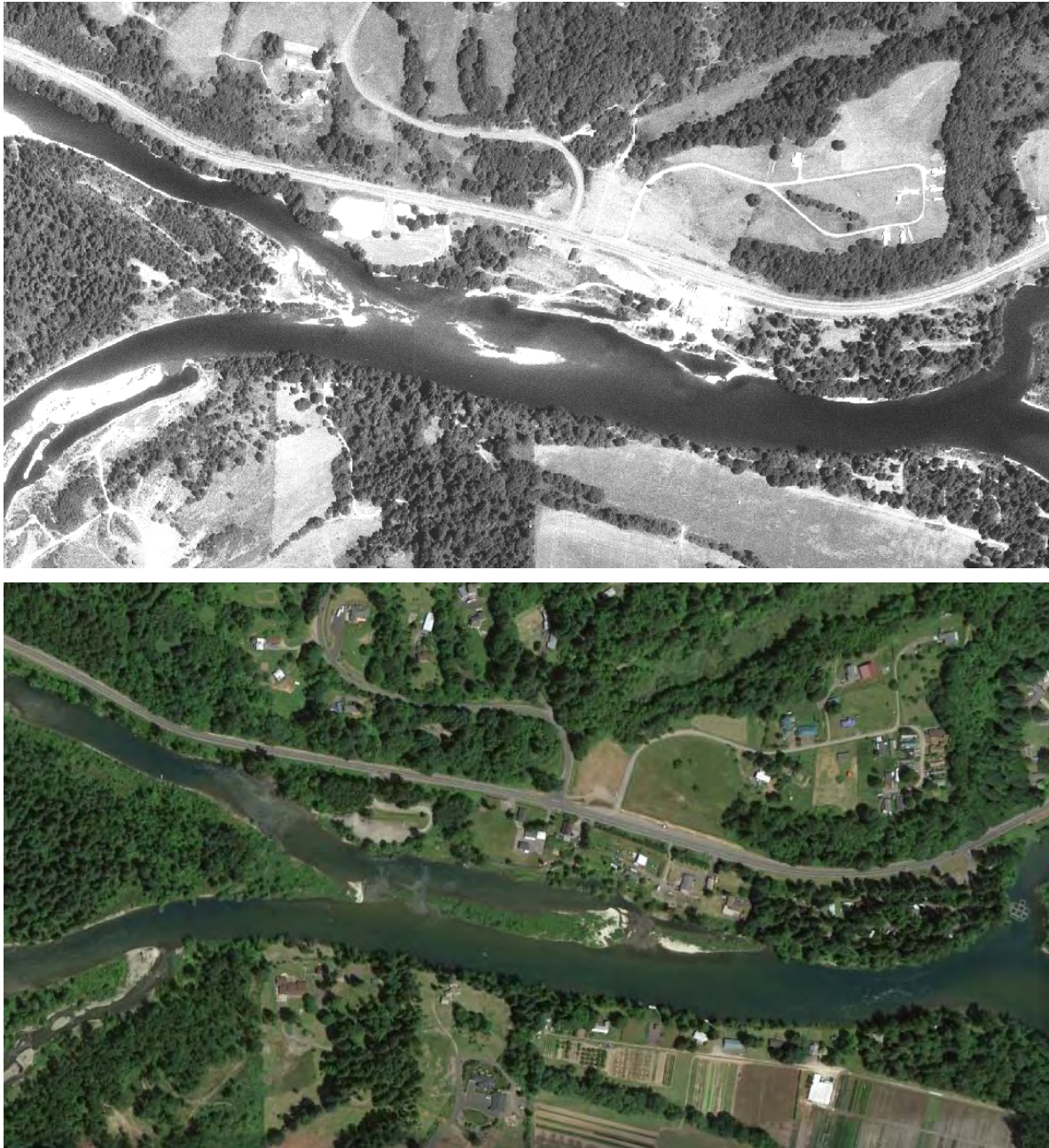
Figure 7. Photos of the top end of Eagle Island in July 1970 (top photo) and July 2012 (bottom photo). Note difference in accessibility of North Channel to fish and the decreased likelihood of adequate attraction flows for fish entry into the North Channel. This effect would be diluted during the higher outmigration flows in the spring, but would nevertheless have some effect on fish usage of the North Channel.
