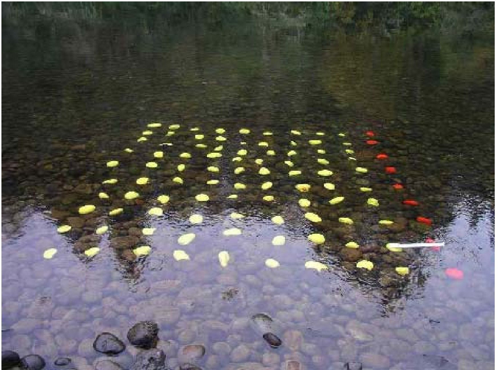
Figure 2. Example of tracer gravel grid.
