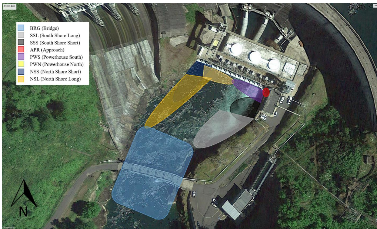
Figure 4. Locations of detection regions for 8 radio receivers located from the bridge upstream and into the fish passage facilities at Merwin Dam.
