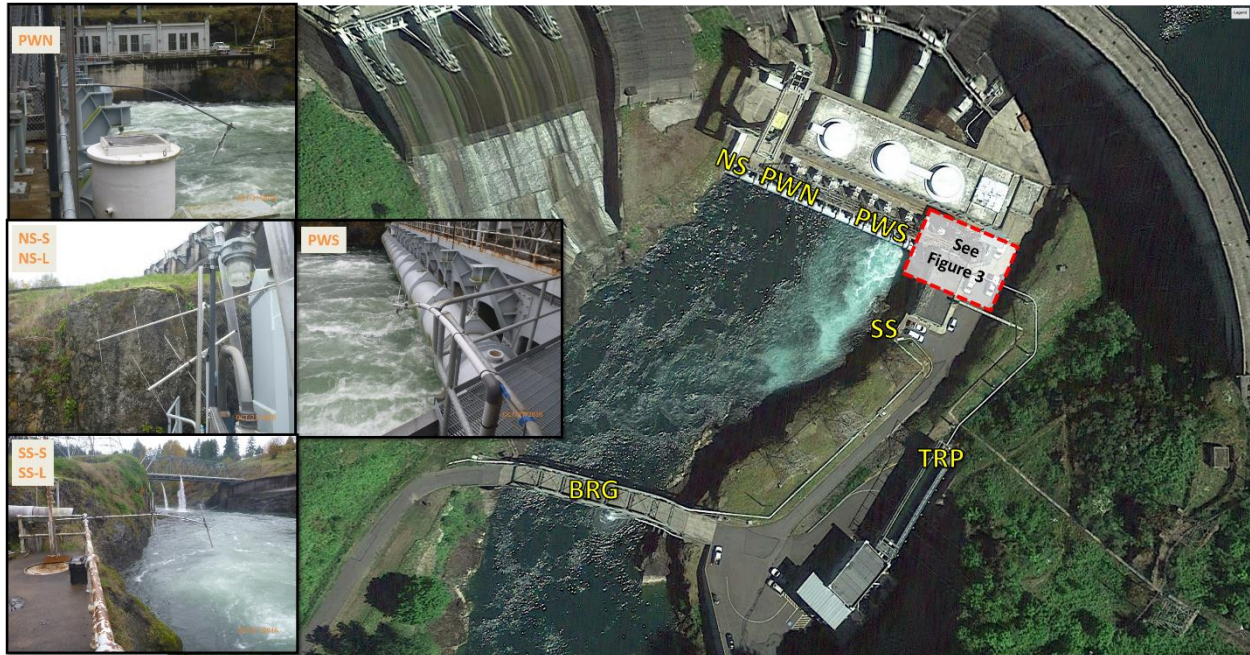
Figure 2. Merwin Dam tailrace area with locations of stationed RT antennas and pictures of select antenna orientations. All RT antennas listed in this figure are aerial, except for the Trap. Details of antennas deployed within the trap are shown on the trap schematic in Figure 3. North Shore and South Shore sites comprised two receiver stations each: one each of a short three -element and a long eight-element antenna. These were designed to cover larger areas along the full shorelines from the location where they were deployed (indicated by icon placement) all the way to the bridge. The bridge array (Bridge) comprised four amplified three-element aerial antennas hung equidistantly across the length of the bridge. Receivers North Powerhouse Wall and South Powerhouse Wall comprised one three-element antenna each, pointed towards the powerhouse and angled slightly down.
