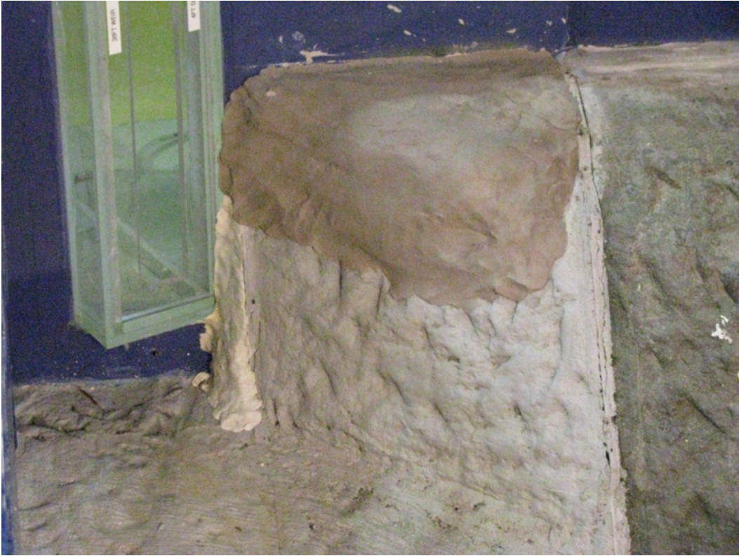
Photo 4.5 Clay Fillet used to Eliminate Left Bank Local Eddy.
