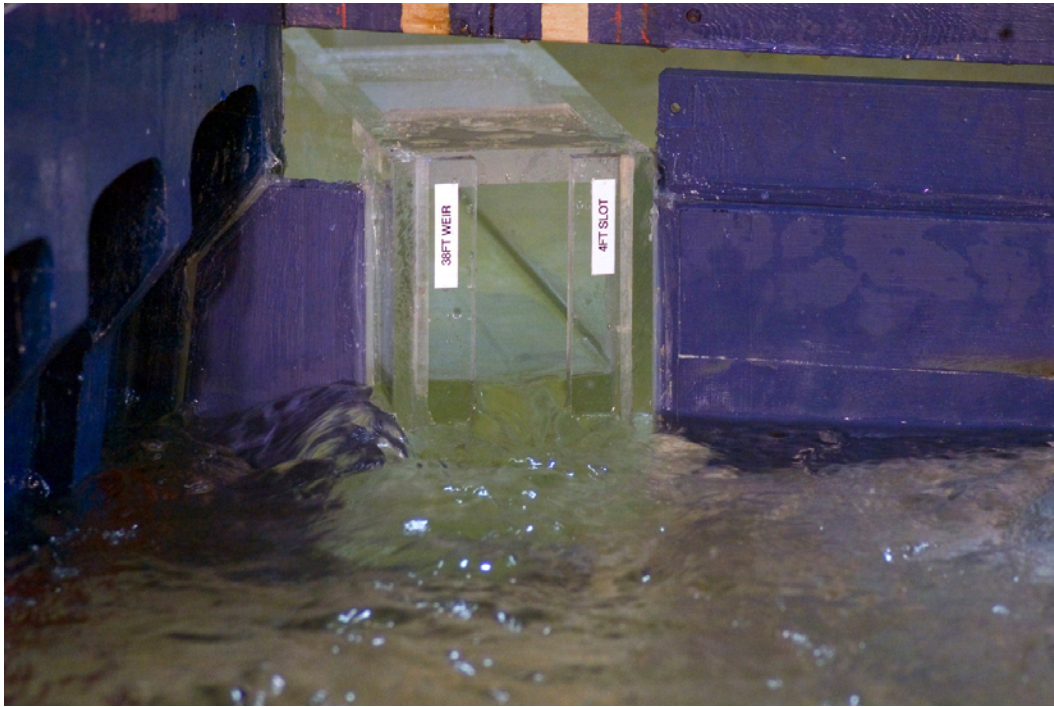
Photo 4.3 Corner Entrance Without Fillet Concept – Corner entrance operating at 400 cfs, 4' wide weir, powerhouse operating at full generation – Looking across from right bank.
