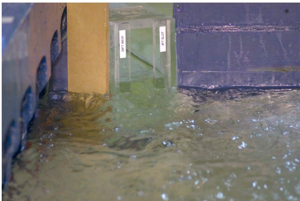
Photo 4.2 Corner Entrance Fillet Concept – Looking across from right bank
