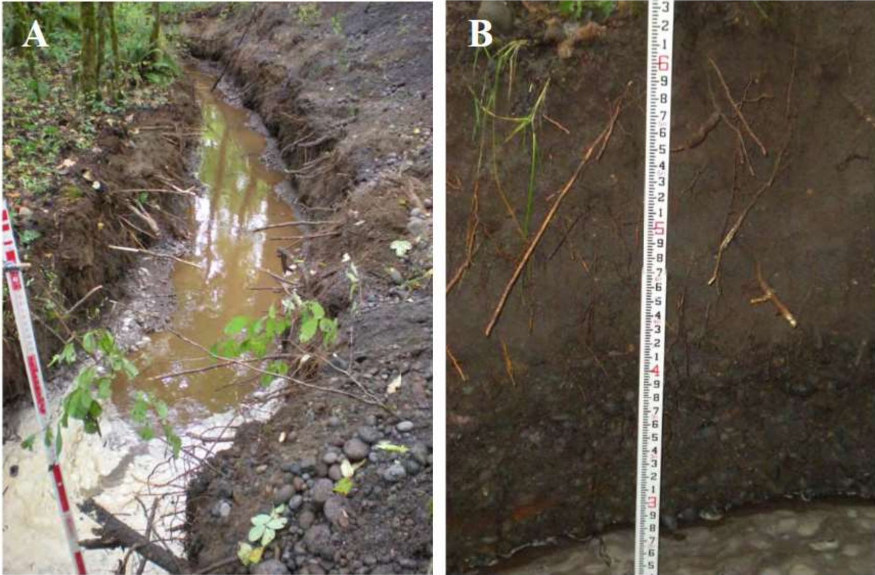
Figure 3. (A) looking upstream in the trench during the pump test. (B) The transition from soil, to sand, and finally alluvium can be seen in the wall of the trench.
