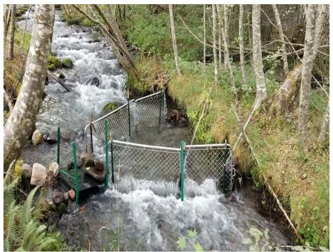
Figure 3.4-2. Swim-thru box and V weir deployed within P8.
