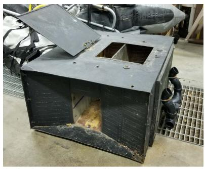
Figure 3.4-1. Swim-thru box that housed underwater video camera.
