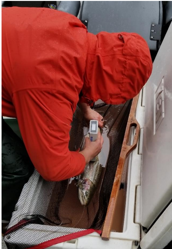
Fatmeter being used to measure muscle lipid content on a winter steelhead. Photo by Chris Karchesky
