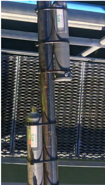
Appendix Figure A.5. ATS reference beacons attached to steel pipe for deployments in the NTS.
