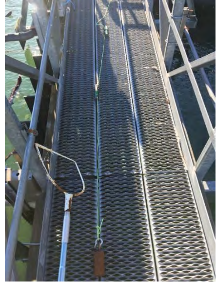
Appendix Figure A.6. Bottom portion of test tag stringer, showing two tags, stringer cord, and weight.
