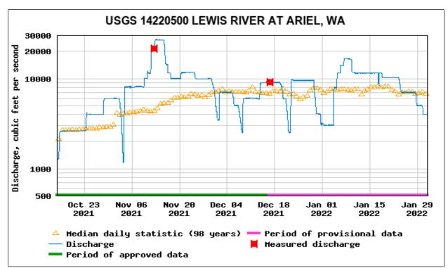
Figure 2. USGS Lewis River Ariel Gage – 15 minute interval reported discharge (cfs) during the 2021 survey season and period of record median daily statistic.
