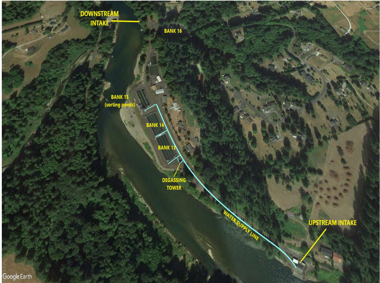
Figure 1. Aerial view of Lewis River Hatchery showing the location of rearing banks and water supply infrastructure
