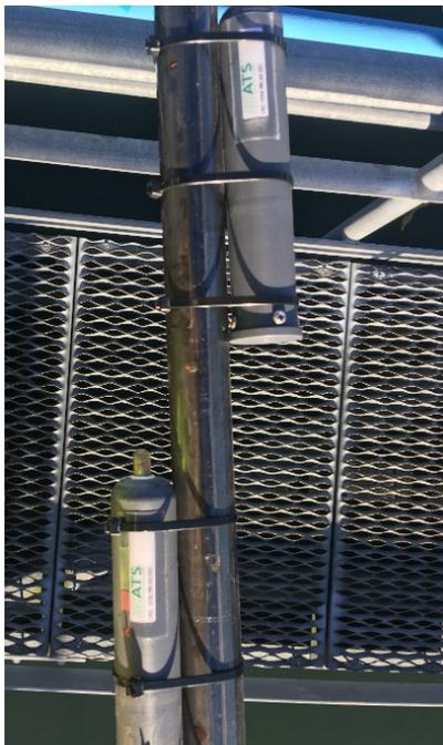
Appendix Figure A.5. ATS reference beacons attached to steel pipe for deployments in the NTS.
