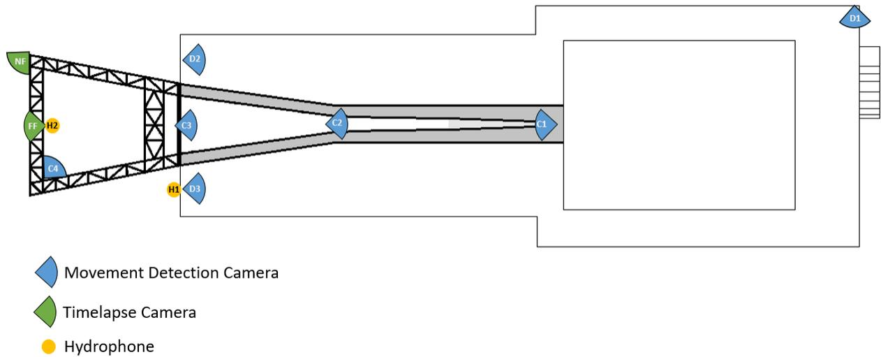
**Appendix Figure A.11. Locations of nine trail cameras and two sound monitoring hydrophones (H1 and H2) deployed on the floating surface collector for the 2021 Swift Reservoir Floating Surface Collector Passage Evaluation.**
