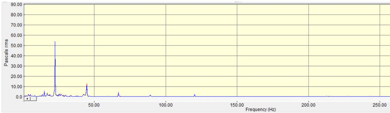
**Appendix Figure B.14. Frequency plot of sound data collected at the upper end of the primary channel of the floating surface collector after the collector was turned off.**
