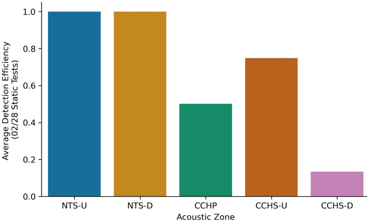
**Appendix Figure A.8.** Example of detection efficiency results from static testing in the net transition structure and collection channel on February 28, 2021. Values depict the average detection efficiency across test tags deployed at various depths in the channel.
