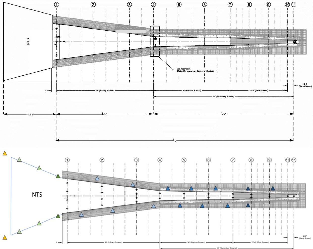
**Appendix Figure A.1.** Swift floating surface collector schematic diagram, showing plan (overhead) view of the collection channel, including primary screen and secondary screen zones.
