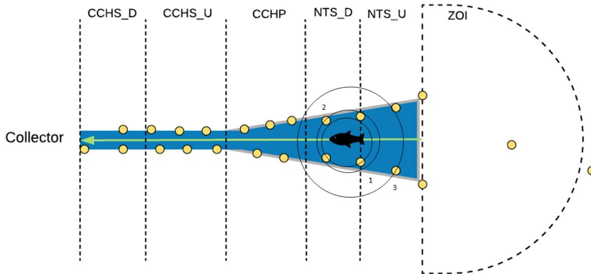
Figure 9. Visual depiction of an acoustic signal being emitted from a tag within a fish and being detected in the net transition structure, primary screen collection channel, and zone of influence. The numbers depict the order in which each receiver picks up the tag signal; in this case, the signal is heard first on NTS-01, then on CCH-01, and finally on ZOI-02. Based on time-of-arrival difference values across these receivers, the tag would be positioned within the net transition structure.
