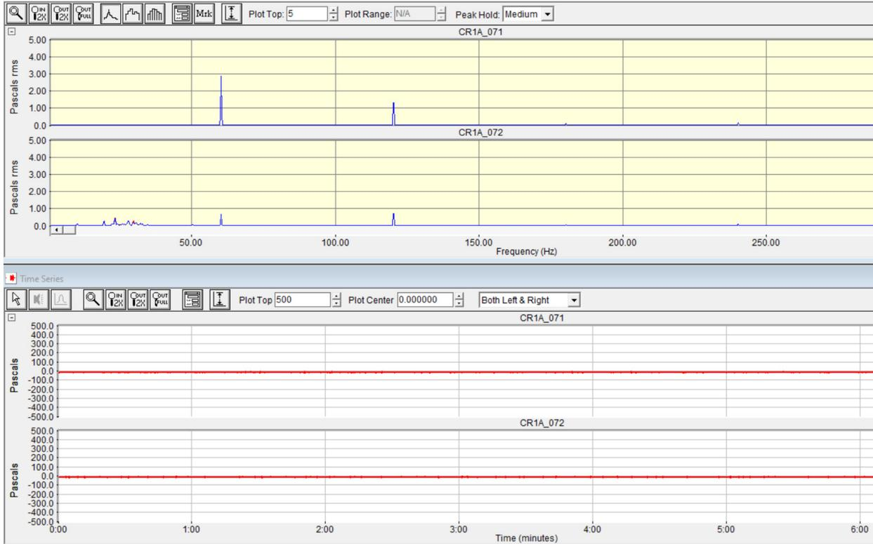
**Appendix Figure B.12.** Sound monitoring plots for the floating surface collector after the collector was turned off at the end of the season for both hydrophones deployed on the floating surface collector.
