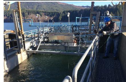
**Appendix Figure A.7. Deploying test stringer by hand within the floating surface collector collection channel.**
