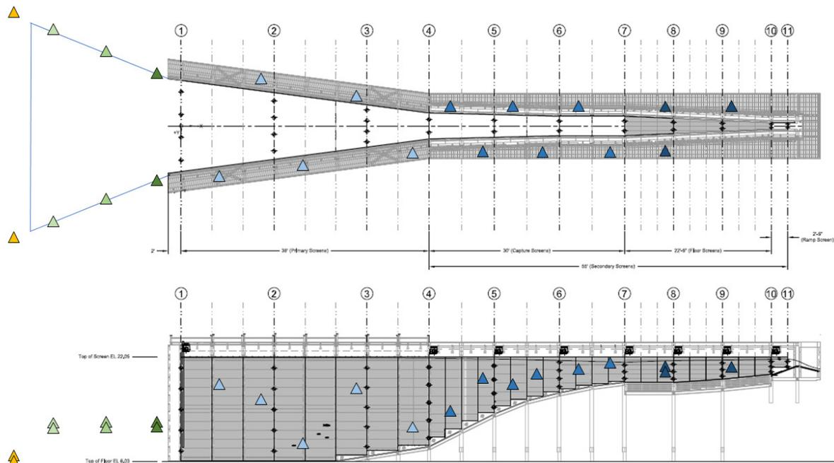
**Figure 8.** Swift floating surface collector schematic diagram, showing plan view (top) and longitudinal cross-section (bottom) of the collection channel. The net transition structure is shown with blue lines in the top plan view, and approximate locations of hydrophones are shown as triangles. Colors correspond to zones listed in Figure 7.
