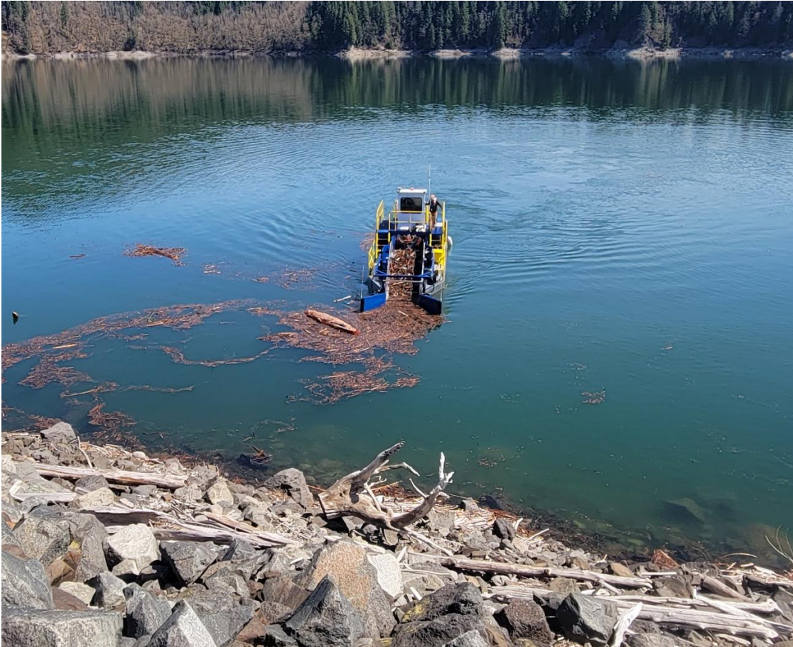
Figure 2.1-3. The specialized debris boat that PacifiCorp purchased in 2022 is used to clear the forebay of debris before it can enter the Swift FSC.
