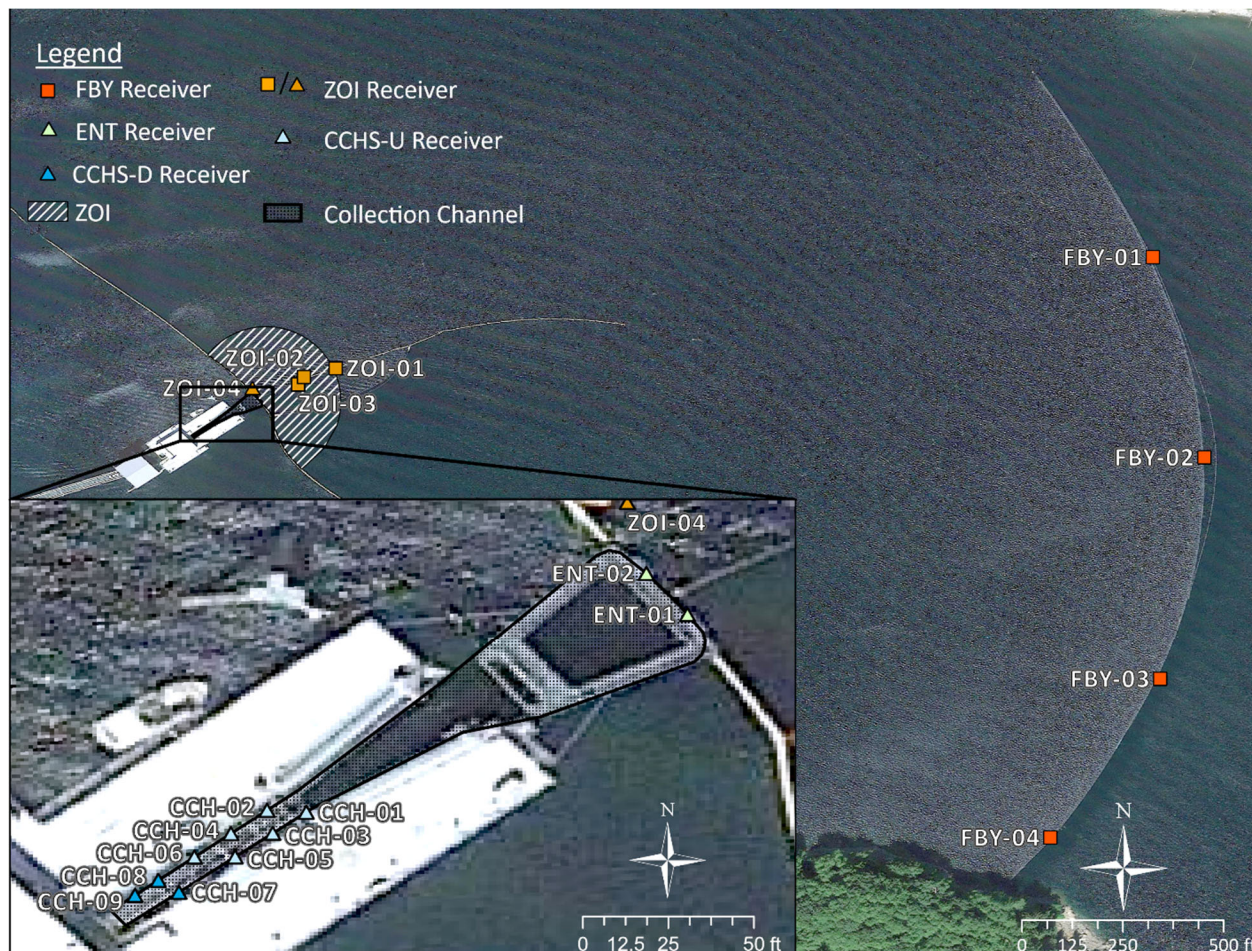
Spatial Reference: GCS WGS 1984; Aerial imagery source: Google. Additional cartography data sources: ESRI. Map conceived and drawn using ArcGIS Pro. Squares depict SR3001 autonomous receivers while triangles depict SR3017 cabled receivers.
