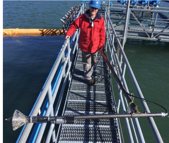
Appendix Figure A.3. Cabled hydrophone and pipe mount. Photo is from 2021 deployment.
