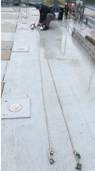
Appendix Figure A.4. Autonomous receivers deployed in the zone of influence, showing rope and shackles that held kettlebell weights. Photo is from 2021 deployment.
