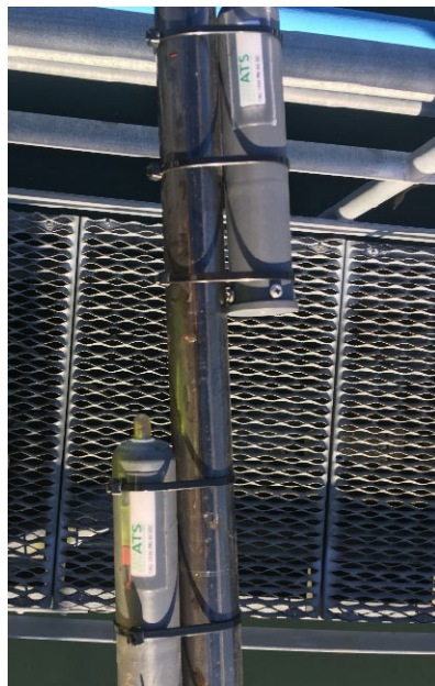
Appendix Figure A.5. ATS reference beacons attached to steel pipe for array deployments. Photo is from 2021 deployment.
