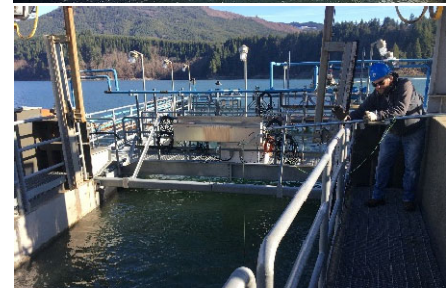
Appendix Figure A.7. Deploying test stringer by hand within the floating surface collector collection channel. Photos are from 2021 deployment.
