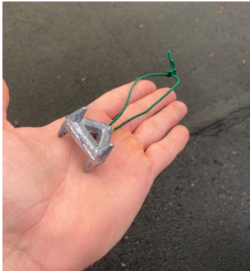
Figure 3.5.1-2. Lead weight and loop that vinyl survey flagging was attached to in 2022 in order to mark bull trout redd egg pockets in the stream in Cougar Creek.
