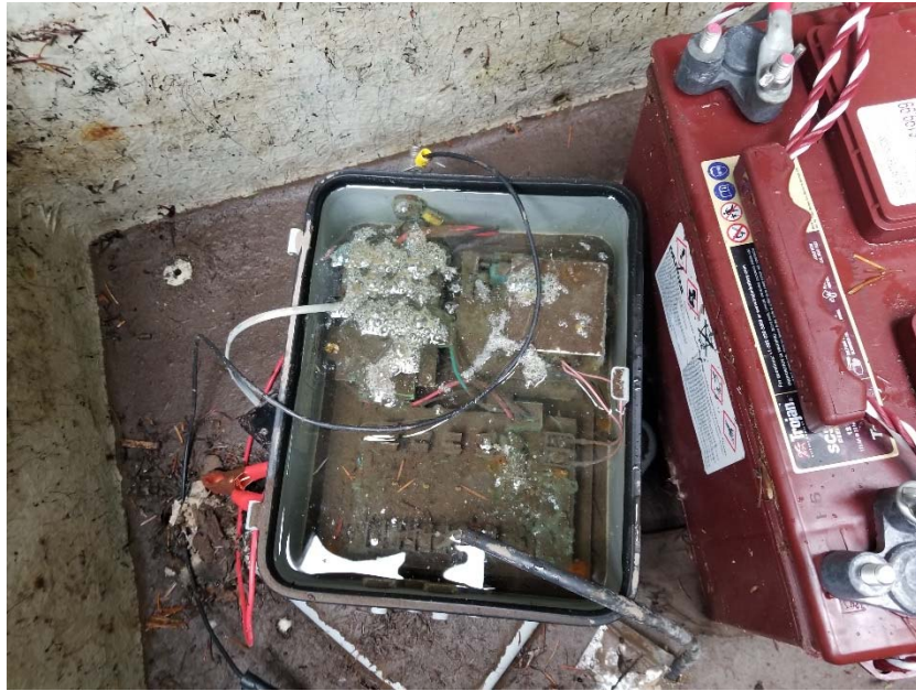
Figure 3.2.1-9. Water damage sustained during October high water event at the Rush Creek PIT antenna site.
