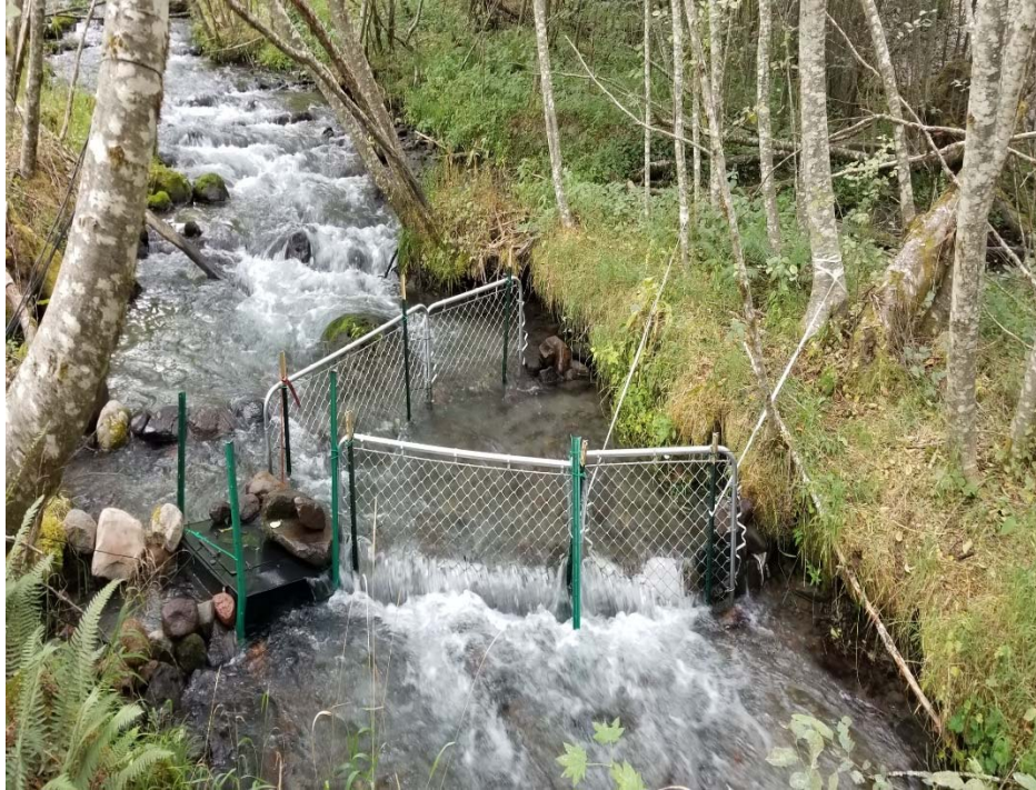
Figure 3.4-2. Swim-thru box and V weir deployed within P8.
