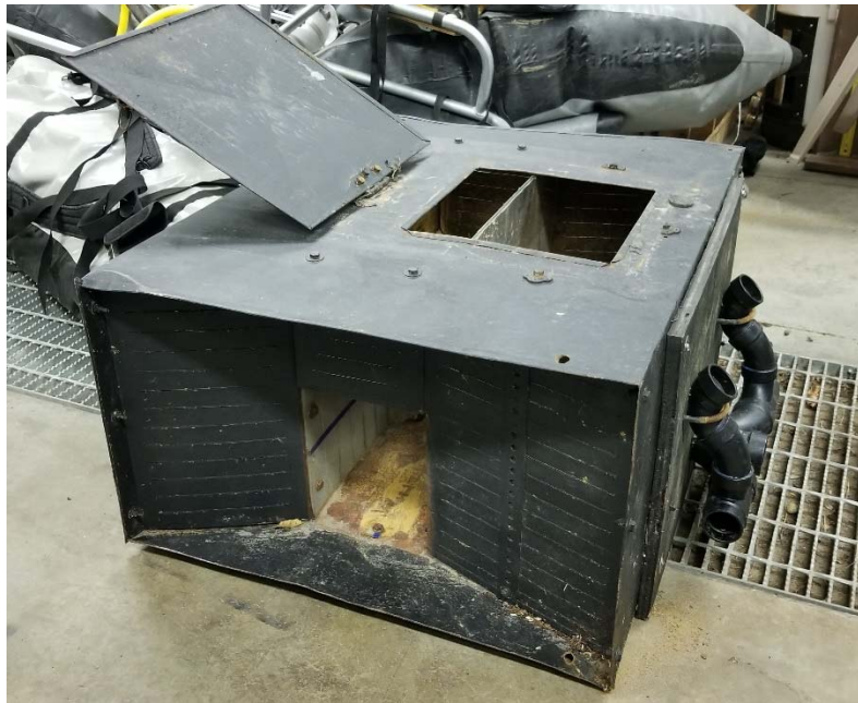
Figure 3.4-1. Swim-thru box that housed underwater video camera.
