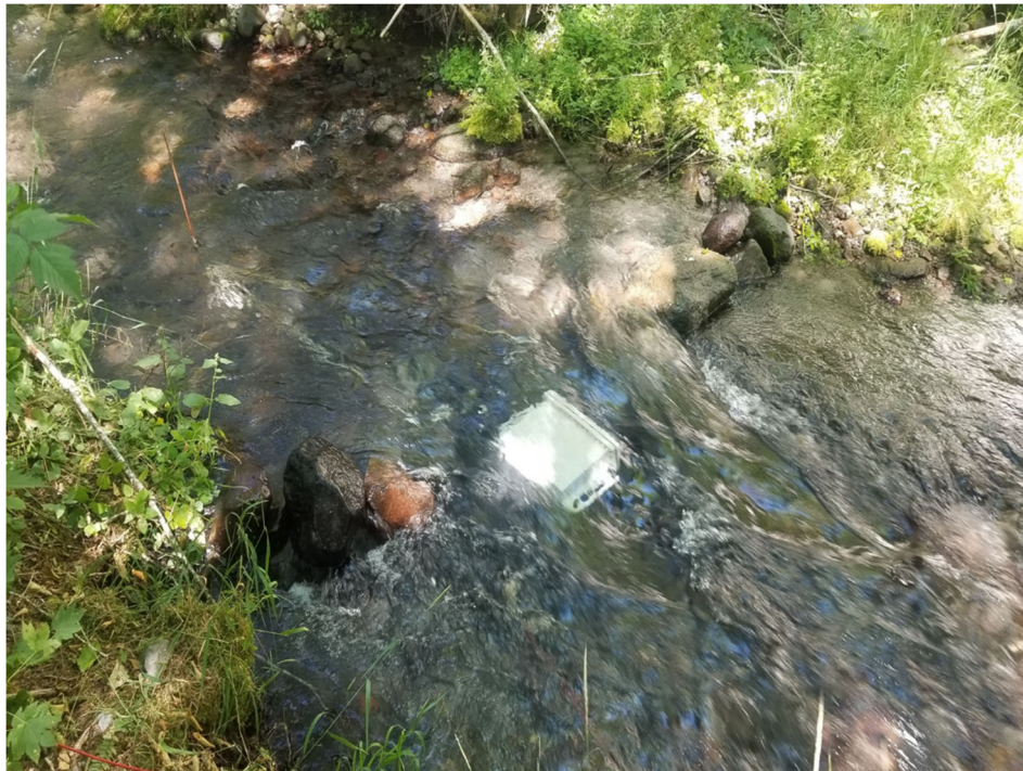
Figure 3.2.1-1. Wagon wheel PIT antenna in operation at Pine Creek tributary P8, 2020.
