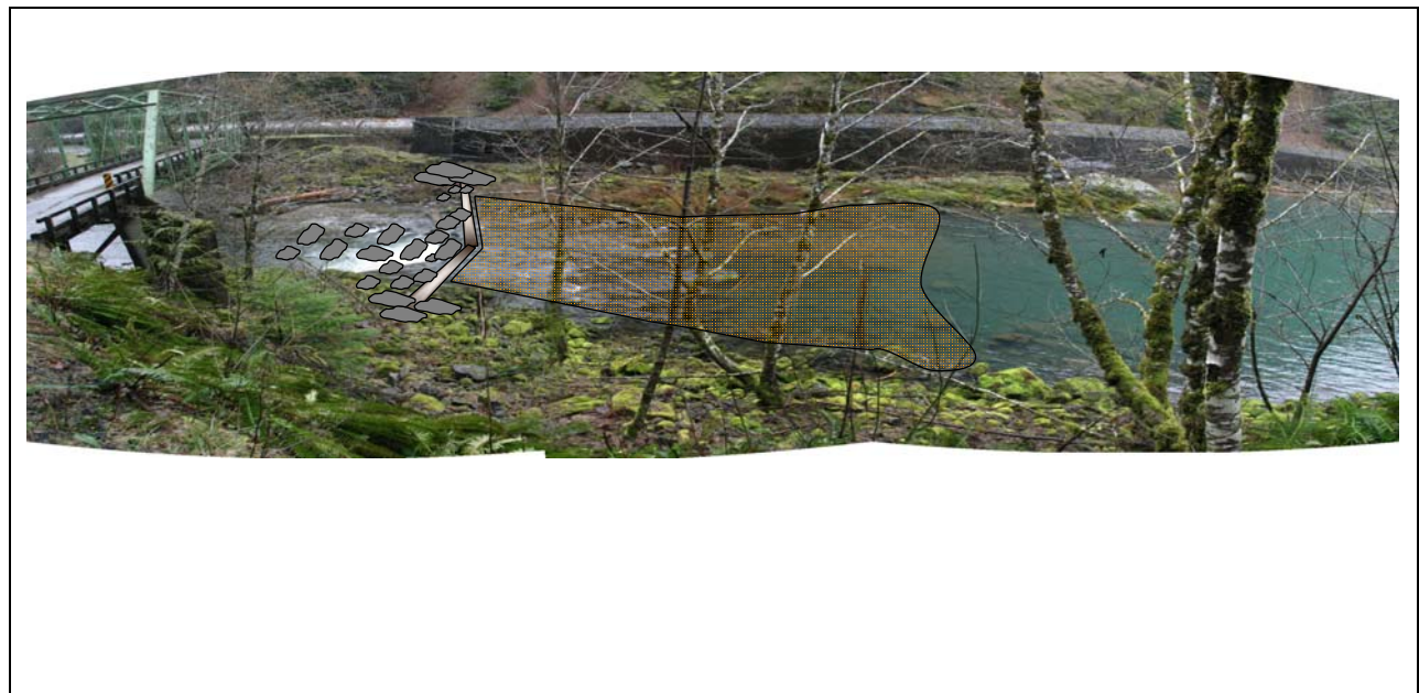
Figure 9. Upper pool tailout showing proposed new log weir, boulders, and area of gravel placement (orange area).
