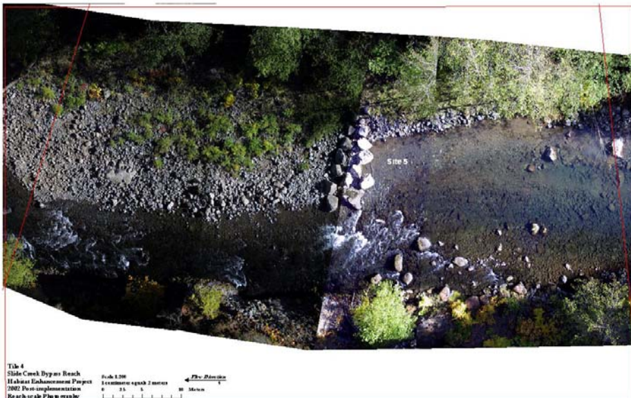
Aerial photograph of a completed salmon habitat project, showing boulders added to trap spawning gravels
