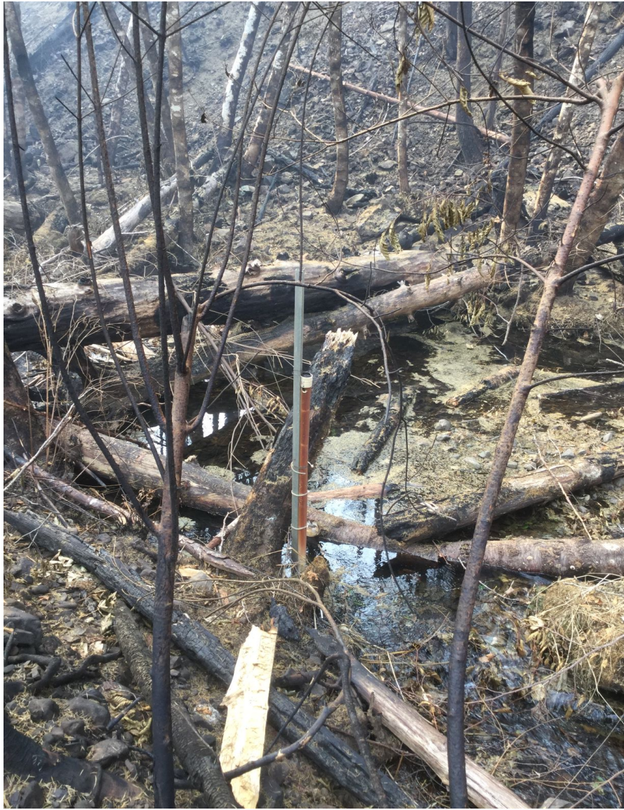
Figure 7. A water quality station that was undamaged by fire on the outside, though the electronics on the inside were destroyed by the heat.
