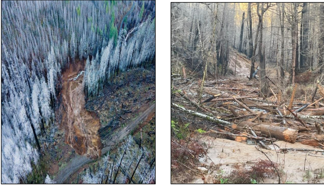
Figure 14. Massive upslope failure on Stoney Creek plugged a culvert and resulted in observable turbidity impacts to the mouth of the North Umpqua River west of Roseburg.
