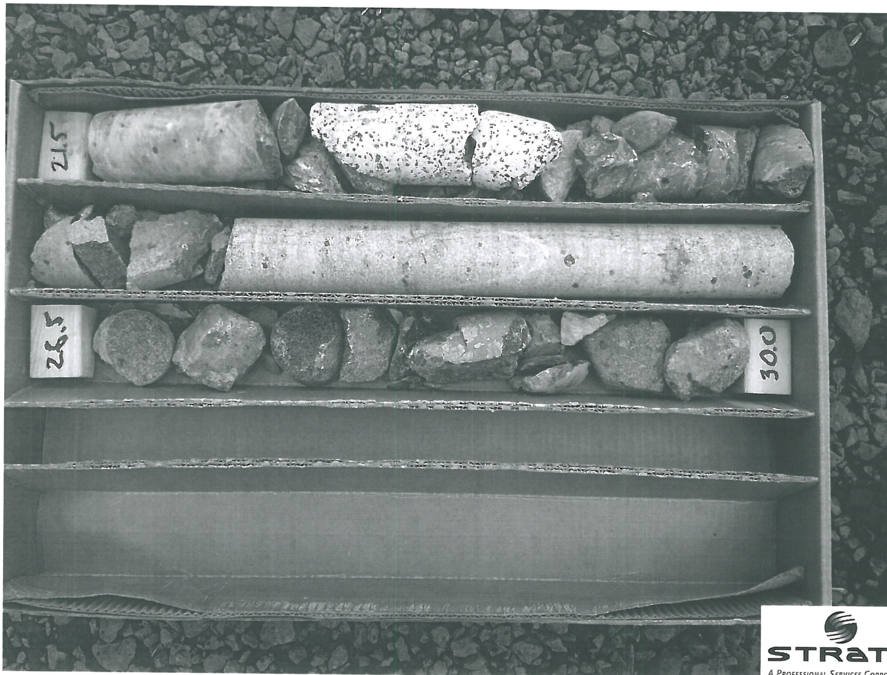
Boring B-2 : Rock core retrieved from 21.5 to 30.0 feet BGS.
