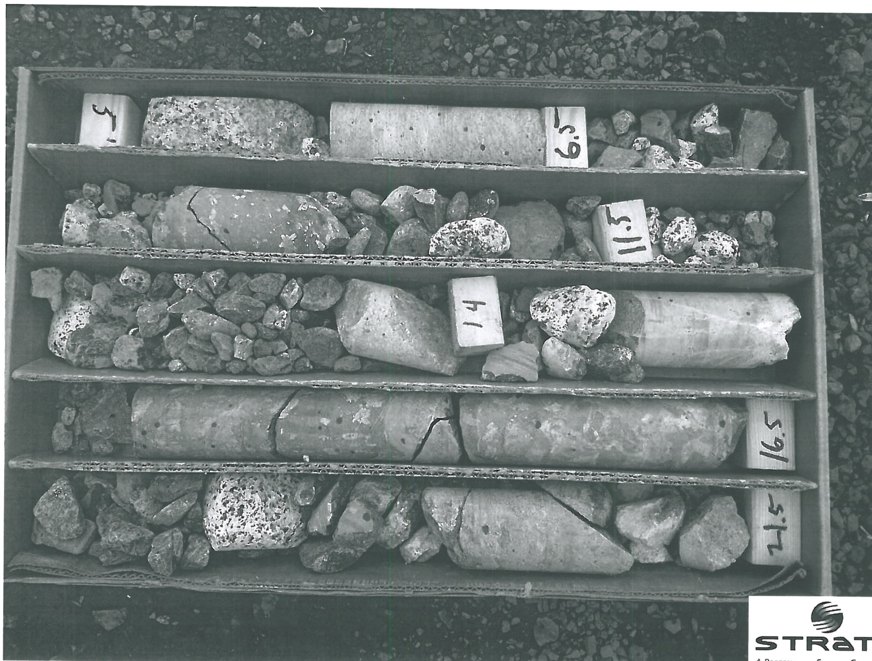
Boring B-2 : Rock core retrieved from 5.0 to 21.5 feet BGS.
