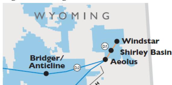
The 2023 preferred portfolio includes the Energy Gateway West Subsegment D.1 project which consists of a new 230 kV line and a rebuild of an existing 230 kV line between the Shirley Basin substation in southeastern Wyoming to the Windstar substation near Glenrock, Wyoming. Both transmission lines are currently under construction and scheduled to come online by the end of 2024.
