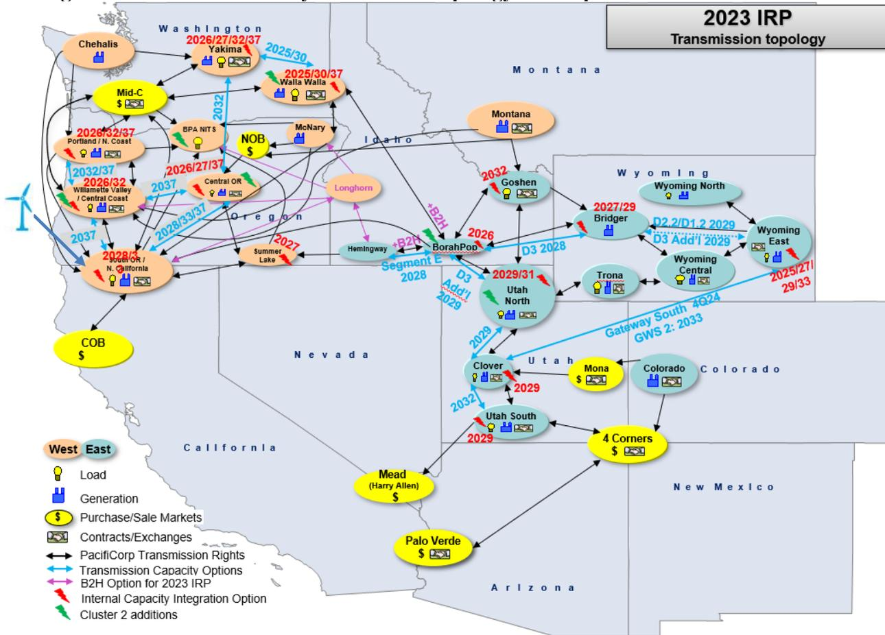
Figure 8.3 illustrates the 2023 IRP modeled topology where each transmission area or “bubble” is defined by any load and generation capability, it’s location on the system and its connections to other bubbles.
