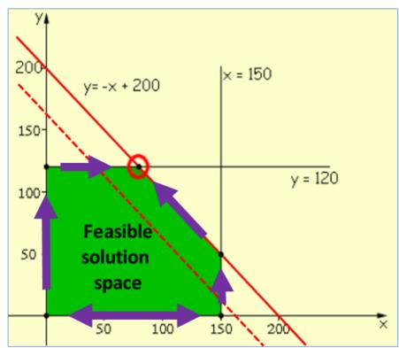
The dotted red line would apply to a scenario where the two generators could not supply the 200 MW needed for load. The model would find an optimal solution in the same manner, minimizing the amount of penalty it must pay
